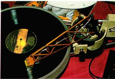
The Sonority tonearm uses a redwood space-frame beam with phenolic headshell and a cast brass base incorporating twin damping troughs.
