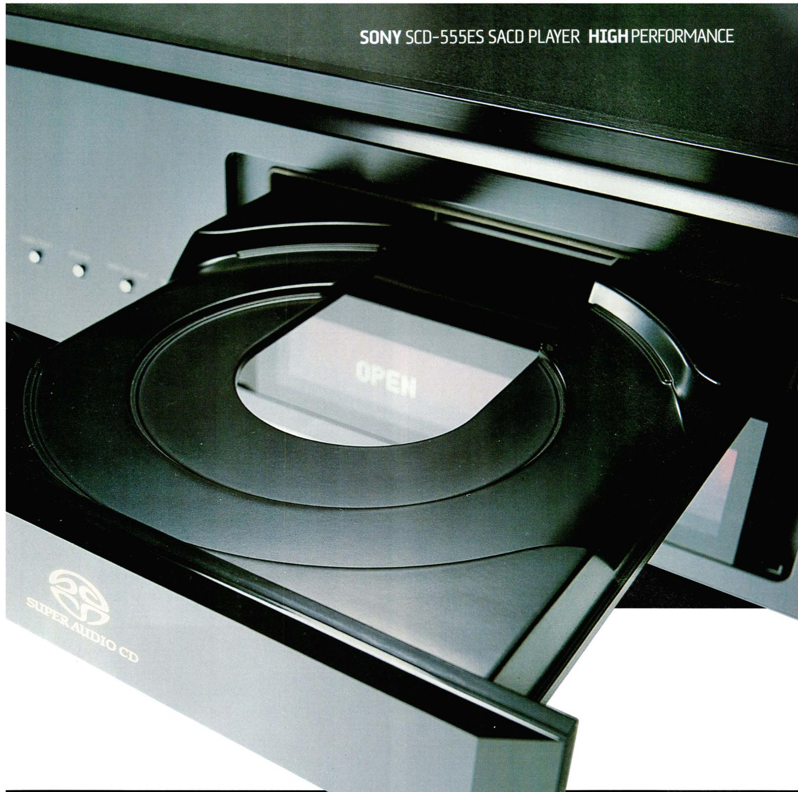
texture takes the SCD-555ES across another technical threshold with distortion as low as 0.0002% at 1kHz/0dBfs, just 0.0004% at -10dBfs and 0.0015% at -30dBfs. The 110dB S/N ratio is short of the potential for SACD but still offers sufficient range for blistering dynamics.
