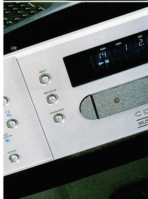
The casework is extremely substantial, with proper screw-together extrusions providing fine mechanical rigidity. The brushed alloy fascia feels as solid as it is strokeable.
