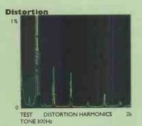
Fig 2 - High amounts of both second and third harmonic distortion.
