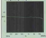
Fig I - Falling treble in frequency response.
