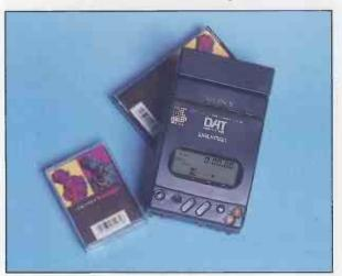
technological wonder draws a lot of current (220mA) to keep its operating solenoids energised. Current consumption increases to a maximum of 400mA when recording with the light on (8mA extra). Even the lid unlocks automatically when Eject is selected. Out of sheer necessity Sony fit a power off switch.
