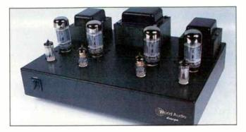
Here's a superb, Class A, 20watt stereo power amplifier that uses the inexpensive Russian 5881 output valve, a military version of the regarded American 6L6, designed for low distortion audio work. It has super-quality output transformers (4/8/16 $\Omega$  selected internally) to minimise distortion and the input stage uses triode working. A rugged, sixteen-gauge, all-welded steel chassis is provided, together with protective bottom plate for safety; a protective top cover is an optional extra.
