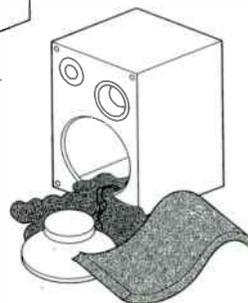
Place the flexible Deflex panel thru' the speaker cut-out and stick to the inside of the cabinet using the recommended adhesive
