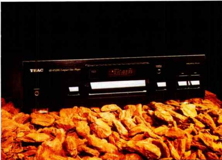
Interestingly it avoids bitstream and its ilk, using instead a 16bit convertor with 8 times oversampling. The new TEAC is well specified, with the usual remote control, shuffle play, repeat and auto-space functions.
