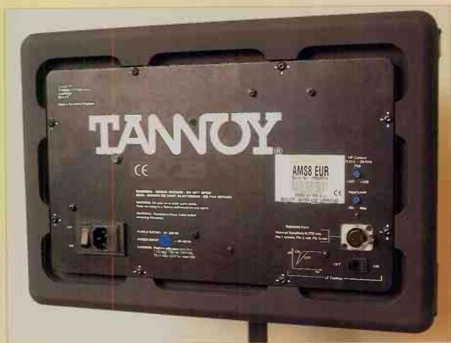
The power amplifier and active electronics are housed behind the metal back-plate. There are controls for treble cut and boost, bass boost and sensitivity.
