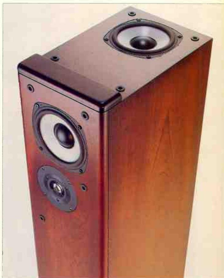
Each of the Harlech's 130mm mid/bass units is loaded with its own quarter-wave horn. The tuning frequency is at 54Hz for the front driver and 78Hz for the top one.
