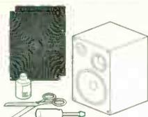
Once you have gained access to the inside of the cabinet, remove foam and/or wool damping from the inside of the speaker (if fitted)
