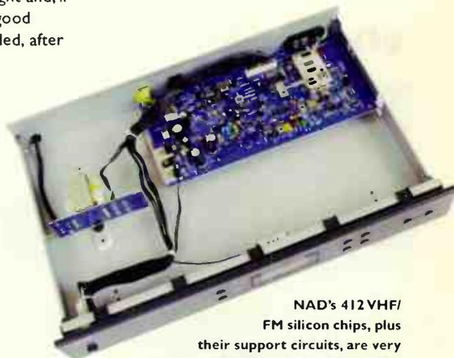
NAD's 412 VHF/FM silicon chips, plus their support circuits, are very well honed by the chip manufacturers. They offer a fine performance, with sufficient stability to need little alignment - and take up little room.
