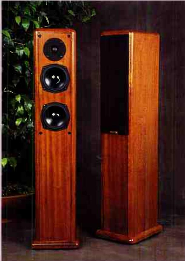
While one of the loudspeaker's two reflex loaded 130mm drivers covers mid as well as bass, the other only works up to about 150Hz, the idea being that two smaller drivers working in tandem produce faster bass with better extension than a single woofer. The rest of the frequency range is dealt with by a 25mm soft dome tweeter.
