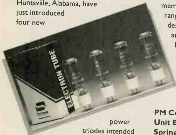
power triodes intended specifically for use in high quality amplifiers. Like the 845 and 211A, these new Svetlanas have direct-heated, thoriated tungsten filaments, but come with massive graphite anodes. Rated at 125w, there's power on tap even in single-ended operation.
