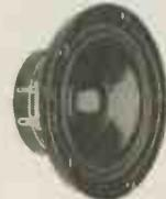
W100S 10cm (4") Low/Midrange. Coated paper cone, rubber surround, high temperature voice coil. Suitable as woofer in mini enclosures or midrange in 3-way systems. 4ohm. £18.06
