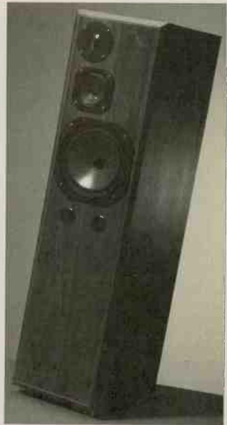
Our KLS6 design uses an open baffle midrange driver to eliminate cabinet coloration. The open cavity is filled with long hair wool to absorb rear-firing energy.
