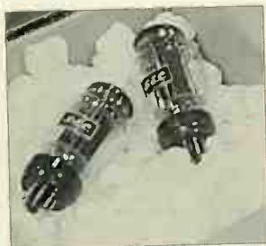
A pair of original GEC KT88 output valves, worth around £60 apiece at least (more in the Far East) - hence the protective packing.
