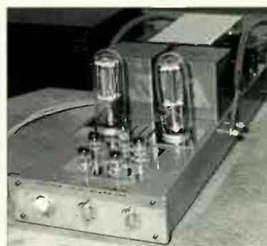
The Menthor 211 stereo 20watt valve amplifier, designed in Japan and produced in Malaysia.
