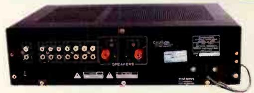
**Plug the cables from the pre-amp into the CD sockets on each A-400 and use, say, the right input and loudspeaker sockets for the tweeter and the left for the mid/bass unit.**
