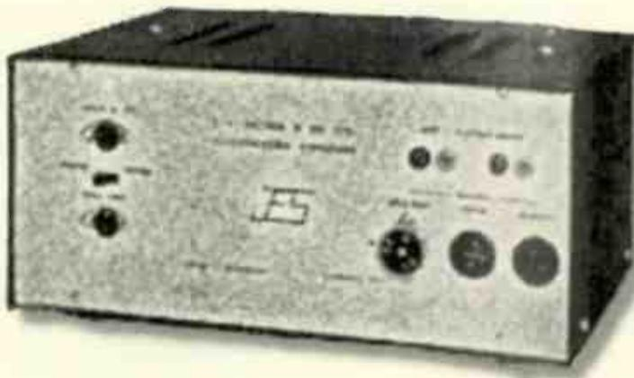
1975's P51 power amp, shorn of the Series Two's heatsinks, produced 50W of class AB power.
