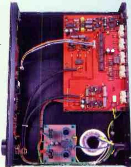
The Hurricane I pre-amp here is fitted with the optional phono stage. This can be adjusted to suit either MM or MC by moving a series of six jumper connectors.
