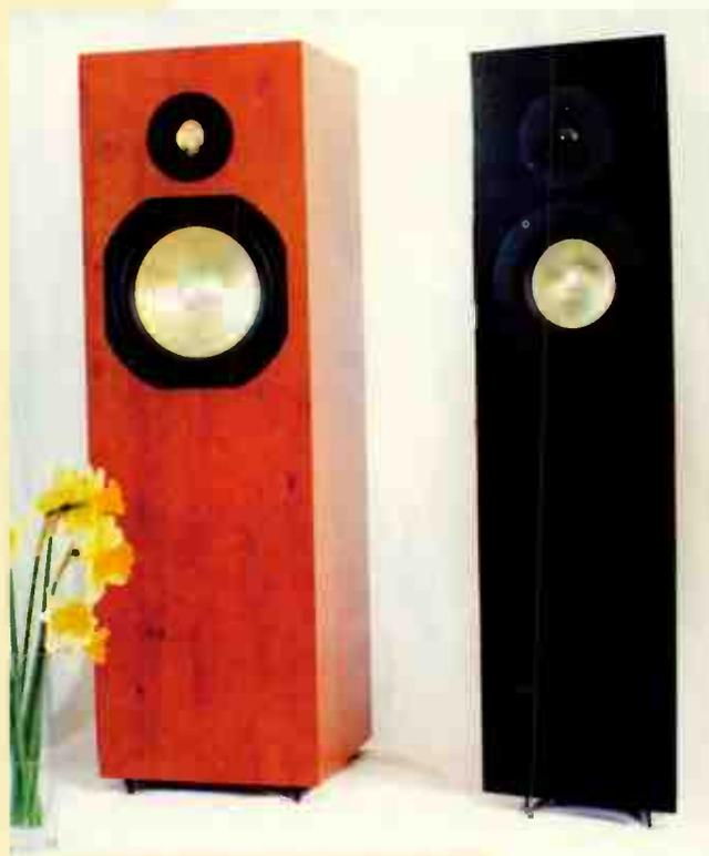
Making up the driver complement for the 300 is Audax's high quality piezo gold dome tweeter and a 180mm mid/bass driver with an anodised spun aluminium cone. This crosses over through a simple, first-order network at 6kHz. With a braced cabinet hewn from 25mm MDF and veneered inside and out, the Concept 300 will set you back £1800.
