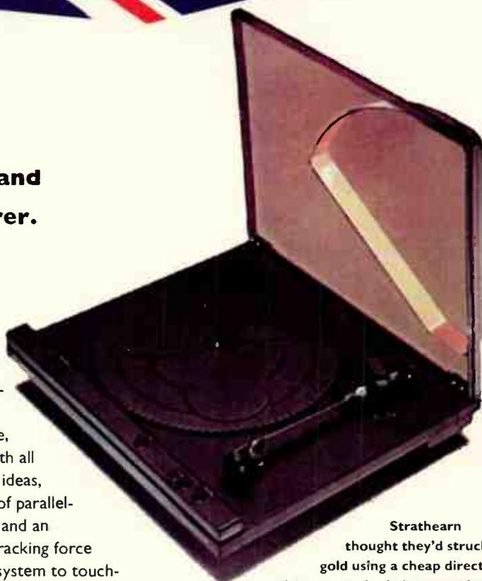
Strathearn thought they'd struck gold using a cheap direct-drive motor in their turntables. Unfortunately the decks rumbled almost as much as tube trains.
