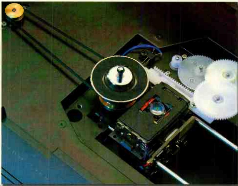
Using Parasound's C/BD-2000 is a bit like using a record deck. Slipping back the smoked Perspex transport cover, you have to put the disc over the spindle and then place the surprisingly heavy puck on top. By the way, don't forget about the puck. The transport works whether it's used or not, and leaving it off can result in the disc spinning crazily inside the machine.
