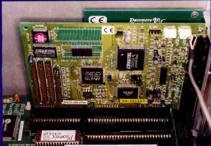
The soundcard fits into one of your PC's expansion slots. Connections provided are Line In, Line out, Speakers and Mic In.
