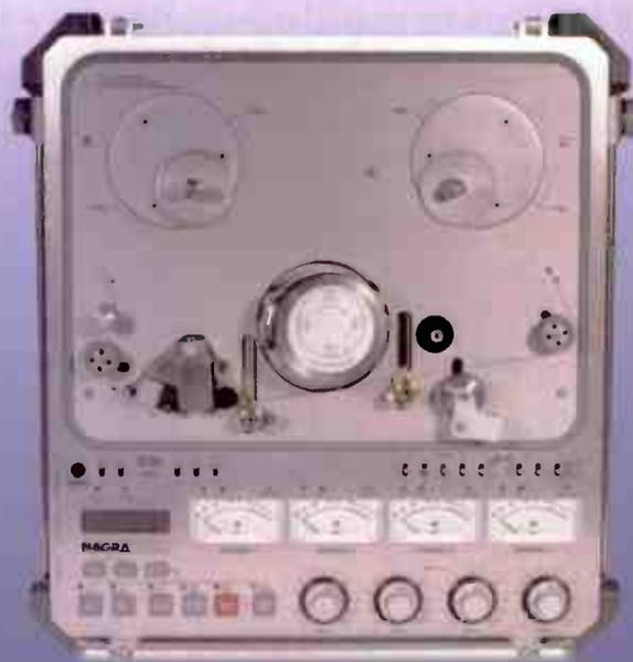
Nagra's D open-reel recorder uses 0.25in. tape with recordings laid down via a VHS video-type head. For longevity's sake, there are few plastic parts or glue joints in the transport and casework.
