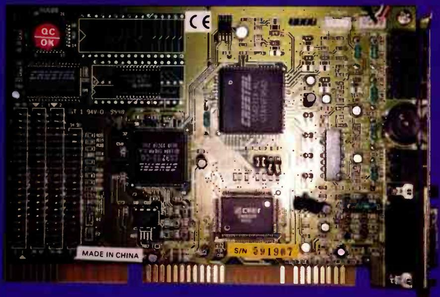
The soundcard itself uses Crystal Semiconductors' chips to provide Analogue to Digital and Digital to Analogue conversion.
