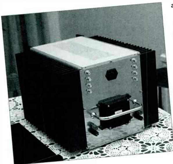
The Class A power amp is made from high-grade components, including a pair of huge heatsinks to keep it running cool (ish!)
