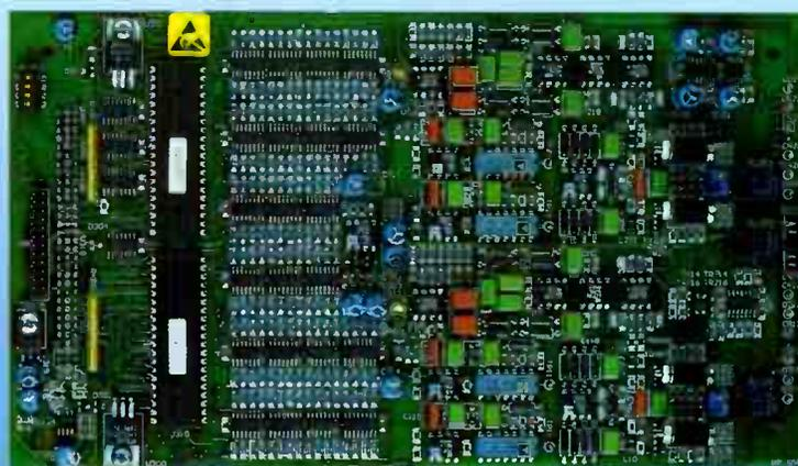
The DAC board from dCS's Elgar converter. The two large chips are Read Only Memories which control how the DAC works. The group of surface-mount chips are current sources; everything to their right is the analogue output stage.
