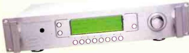
**B&W's Listening Room Optimiser sits between transport and DAC and can create a digital filter to correct room response anomalies. Two benefits are better imaging and sound staging.**
