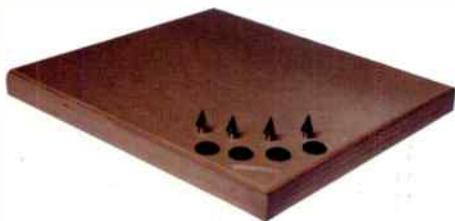
At first sight the Absorber Platform seems like a thick piece of multi-ply wood. Measuring 440mm by 400mm by 36mm it's rather more complicated than it looks. Inside the platform there are 428 individual chambers each of which is 90% filled with small steel balls. The remaining space in the chamber is taken up by fine silica sand.
