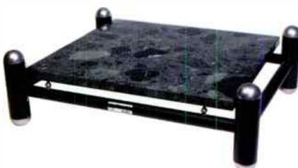
Inside the Monolith's hollow steel frame (595mm by 460mm by 180mm) is a mix of small-diameter lead shot and extremely fine casting sand. This is high-frequency agitated, so there are no spaces left inside the frame. The 20mm thick rubber-damped marble-agglomerate shelf is located on four spikes through four small lead decoupling discs. More spikes in the hemispherical aluminium tube ends lift the Monolith off the floor.
