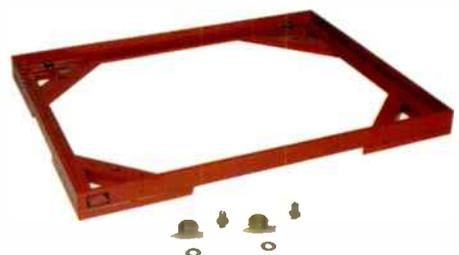
The No Name is one of the simpler platforms here as far as innards go. The outer frame (508mm by 400mm by 50mm) is made from mild steel welded into a rectangle. Four diagonal braces, one in each corner, are filled with SoundBytes (to absorb vibration) and carry the adjustable spikes which sit in brass cups to protect soft surfaces. Four ball bearings mounted on threads allow the glass top-plate to be levelled.
