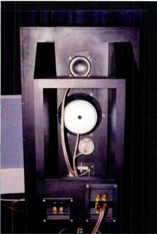
At the rear of the loudspeakers are two binding trays. The one on the left runs direct to the woofer while the one on the right feeds the tweeter/midrange passive crossover.
