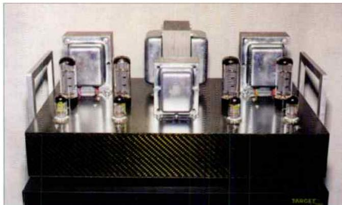
The valve amp's moulded carbon-fibre chassis has the large output and mains transformers bolted to its upper surface, along with the PSU inductor and valves.
