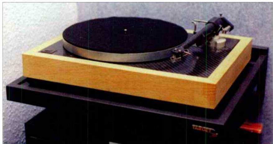
The modified Thorens TD150 uses the original platter, bearing and motor but everything else has been changed.
