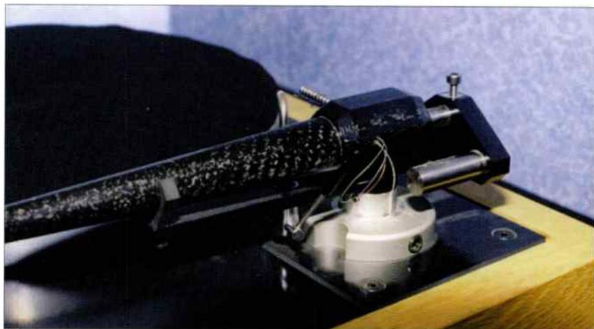
The cabling exits the arm at the pivot point on the prototype. This will be changed on production examples to reduce potential electrical interference.
