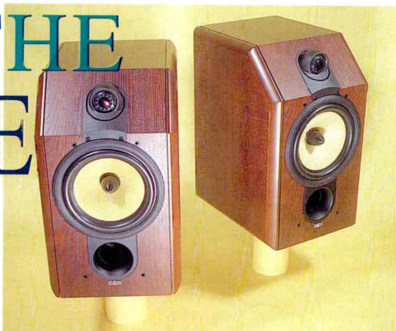
Leo Lam meets the Kevlar mid/bass drivers and metal-dome tweeters of B&W's new CDM1SE loudspeakers.
