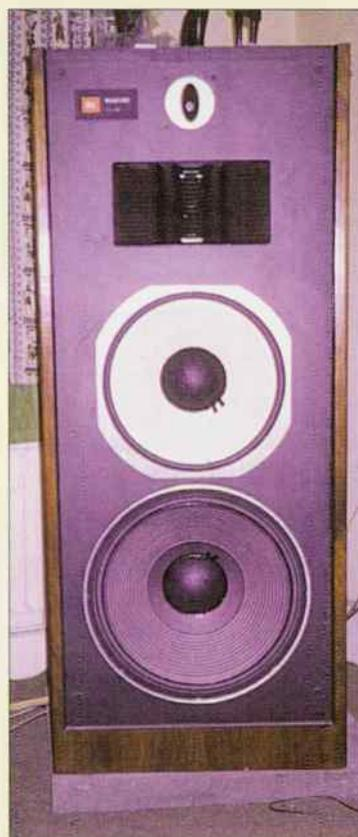
Rey's JBLs load their 14in. woofer with a 15in. passive radiator for fast, clean bass. The midrange unit is hidden behind a slatted diffuser.
