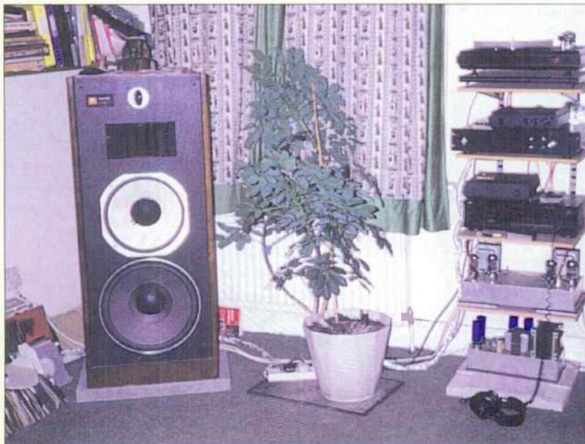
The JBL L220 'speakers sit on concrete slabs to improve the bass. On the shelves to the right are a Pink Triangle PT TOO with battery PSU, Pip I pre-amp (unused), Rey's own pre-amp, a JVC cassette deck, Rey's own power amp and matching separate power supply.
