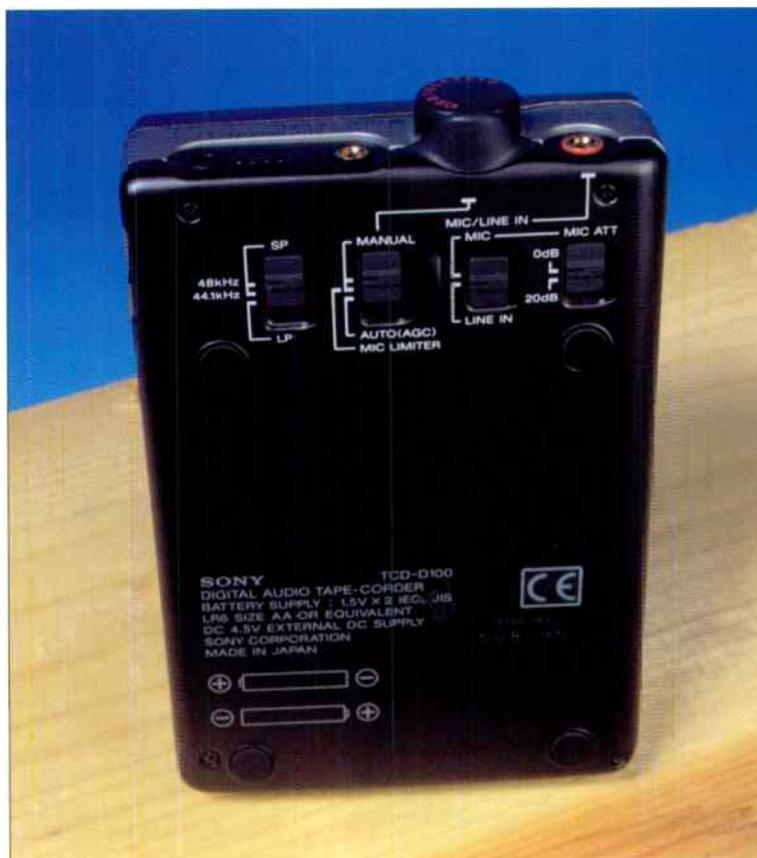
Controls on the TCD-D100's rear include Short and Long Play modes as well as 44.1/48kHz sampling rates. Other options relate to microphone and line inputs.
