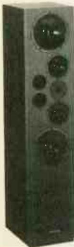
A real heavyweight performer with a total of no less than five drive units in each cabinet. Together these produce a satisfyingly smooth and wide frequency response. The single tweeter is a special 25mm high-end unit with a double coated fabric dome and ferrofluid for cooling and damping. There are two 13cm mid-range speakers and two 20cm long throw woofers for extended bass.
