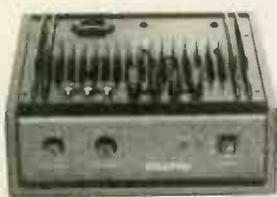
This attractive module consists of a low pass filter and power amplifier ready for you to mount in a suitable sub-woofer cabinet. The combined unit can then be combined with any new or existing hi fi or home cinema speaker system to add in the real bass punch missing from most setups.
