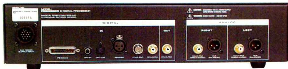
The thin, wide I<sub>2</sub>S-enhanced input joins an impressive array of socketry on the Processor 3's back panel.
