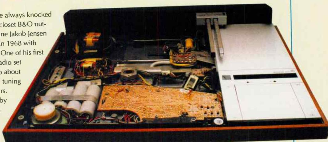
The '4000 has not got a single screw or nut showing on top. To gain access to the deck's innards, a screwdriver has to be inserted into the base and a couple of screws loosened. This releases the wood trim and the aluminium panels atop.
