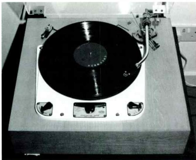
The Garrard 301 motor unit in its Bastin plinth heads up this 'valves and vinyl' system.
