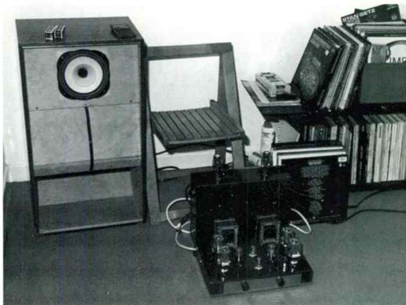
no overall feedback, and produces about 12watts, the same as the single-ended amp mentioned above. The power supply is located in a separate case, and looks as if it might be a little over the top, although I wasn't allowed to peek inside!
