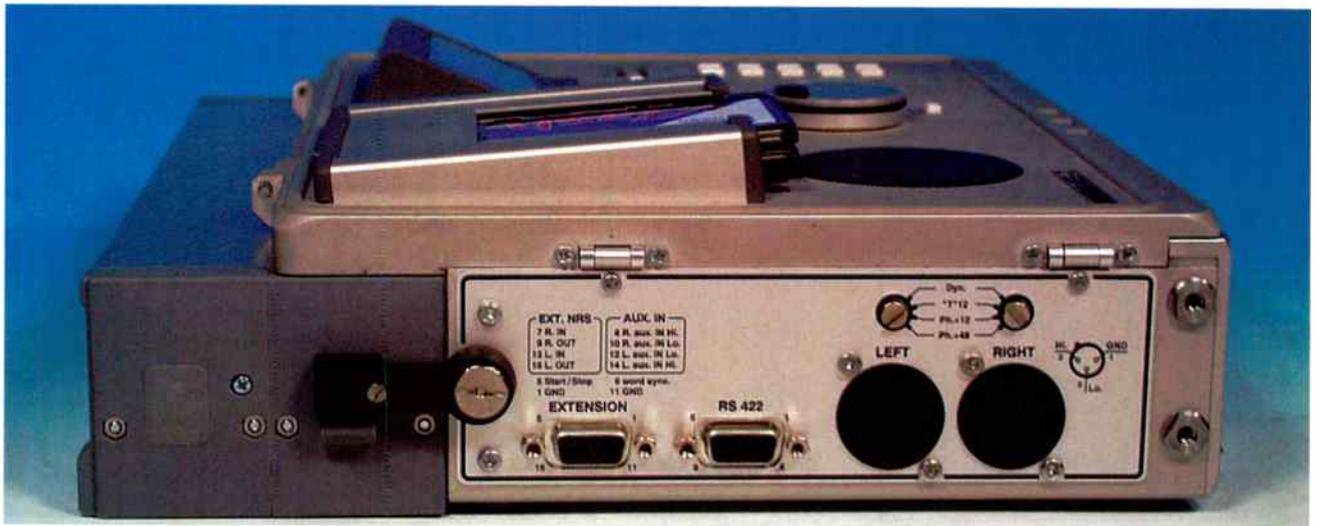
On the Nagra's left side panel are located left and right microphone inputs, the 15-pin line-level input (far left) and the RS 422 socket which allows connection to a PC.
