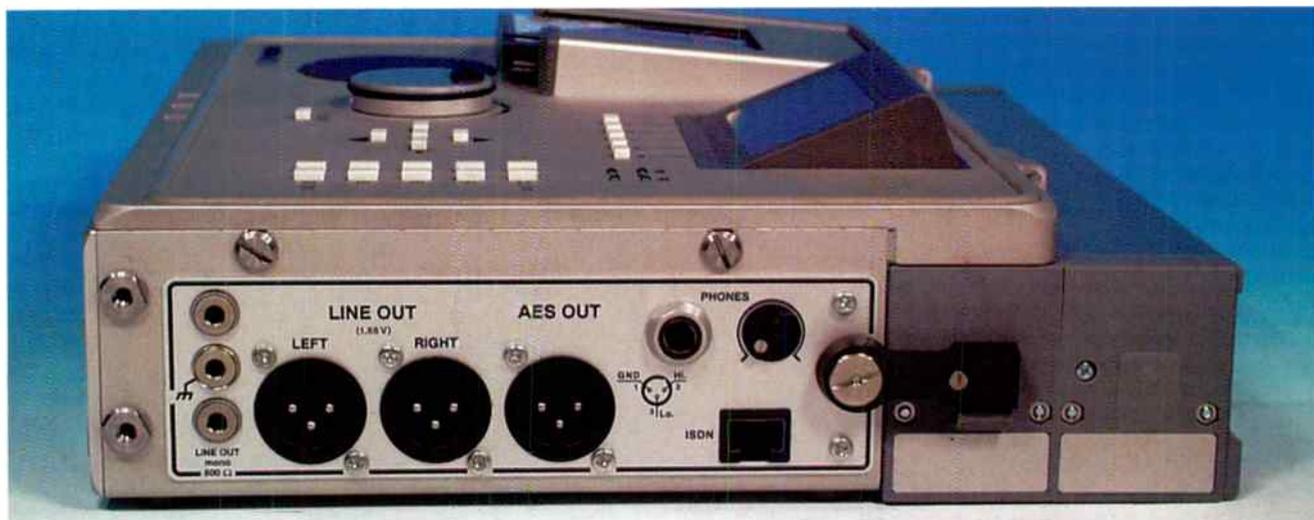
On the other side are the balanced line outs, the AES/EBU digital output, a connector for sending and receiving over ISDN lines and a headphone socket.
