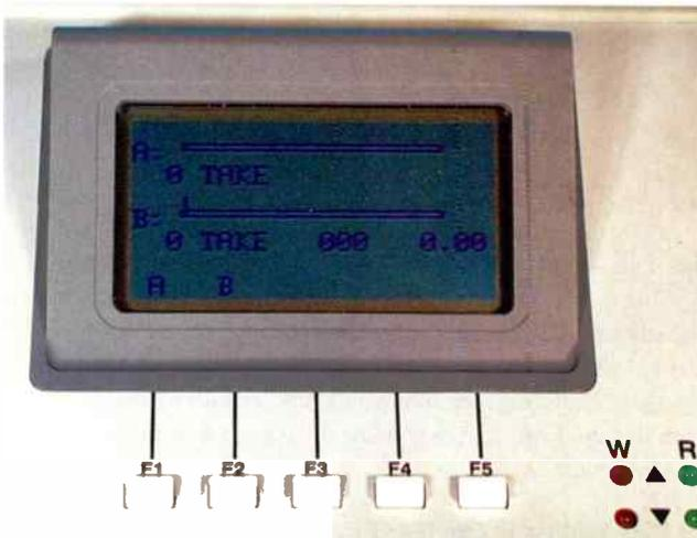
The Nagra has slot-space for two PCMCIA Type II memory cards. You can toggle between these with the F1/F2 buttons. The 'W' and 'R' LEDs denote Write and Read (or Record and Replay).
