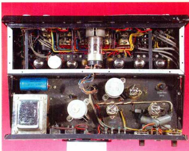
The Empress 556 self-powered pre-amp is a world away from the simplicity of some valve gear. Its plethora of switches and potentiometers can cause lots of noise unless they're properly cleaned.
