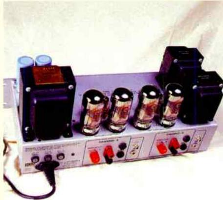
Unlike transistor amps, valve versions need 4ohm/8ohm taps on their output transformers to match loudspeakers of different impedances.
