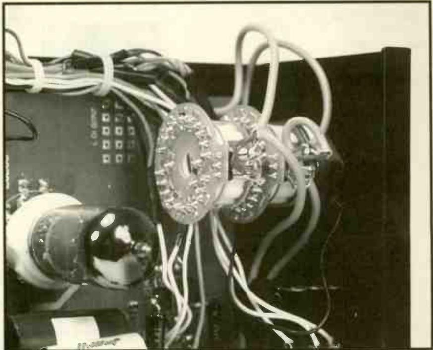
▲ The CT1 uses two Ema switches operating on a pair of small PCBs, which carry the SMD resistors.
