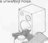
Once you have gained access to the inside of the cabinet, remove foam and/or wool damping from the inside of the speaker (if fitted).
