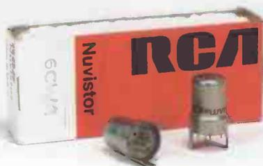
tional valve: no top supports in the form of mica discs; no 'getter'; no glass envelope to melt. At the time of their development it was hoped that power Nuvistors of about 30 Watts would not be long in arriving. What could be more perfect!
