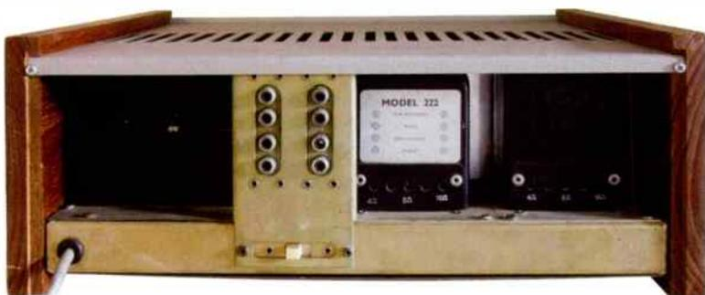
*Basic connections, with two pin speaker sockets.*
