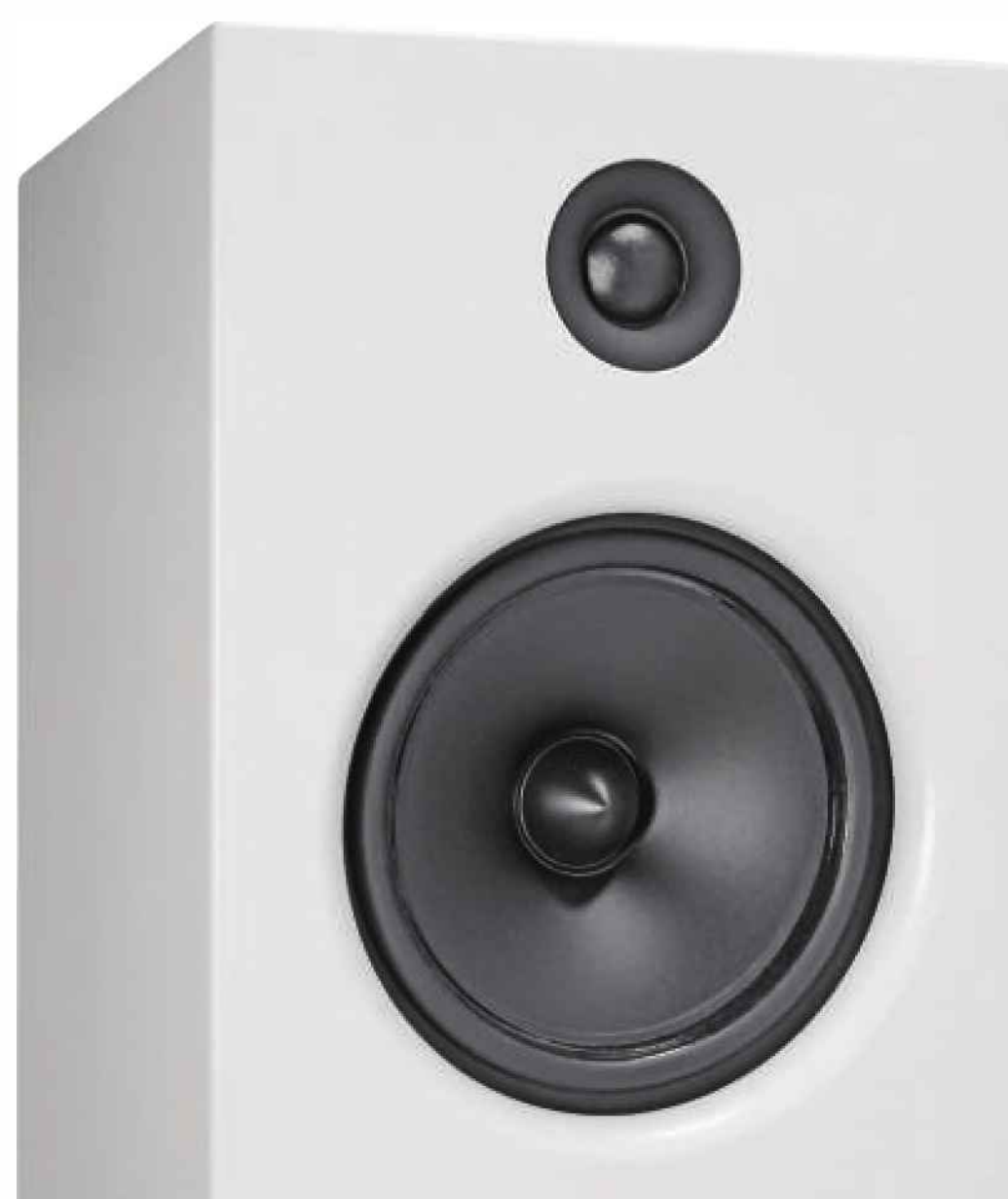
The 25mm soft dome tweeter is housed in its own short-horn faceplate which is said to reduce refraction distortion and give a more even on-axis response.
