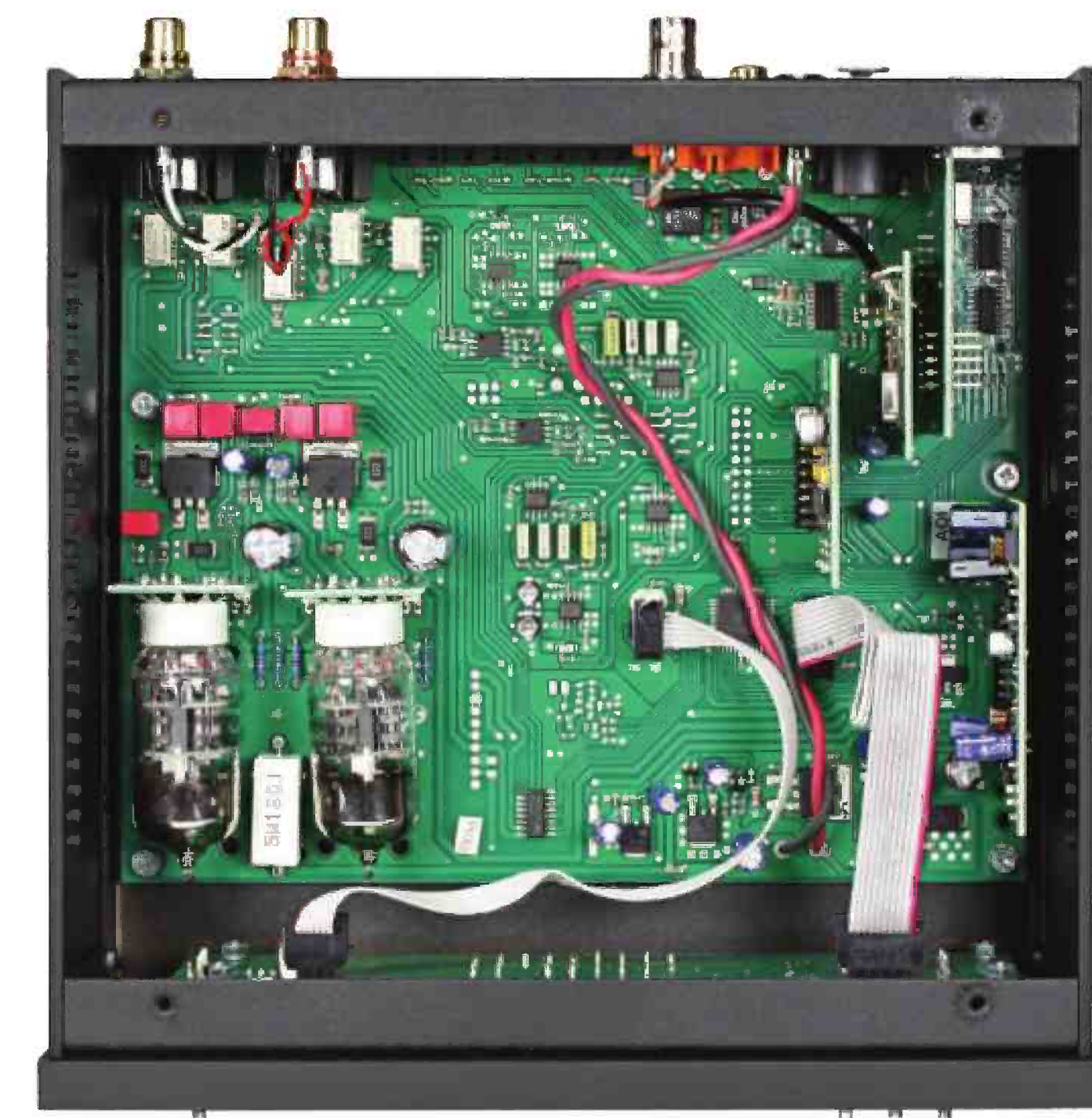
The DAC Box RS' neat internals, revealing its 'motherboard/daughterboard' construction. The USB interface and the PCM1792 DACs account for two of these daughterboards.
