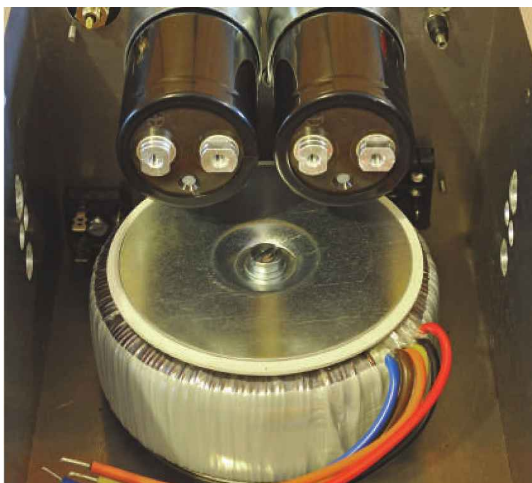
Big 44,000µF power supply capacitors and sturdy 500VA toroidal mains transformer help provide "pile-driver bass with superb grip and control".
