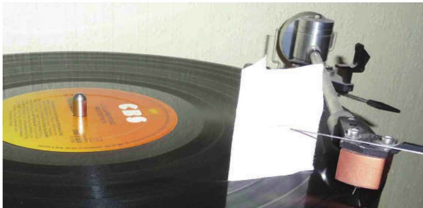
Align azimuth using a pencil lead and sheet of paper, says Alasdair Beal.
