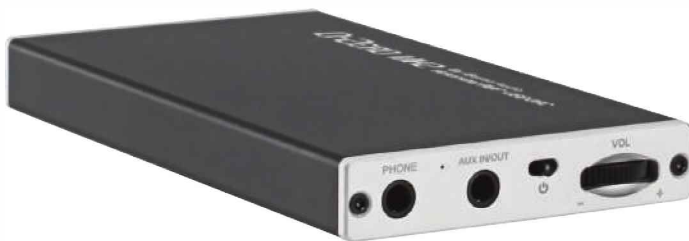
The front of the iBasso contains the rotary volume control, headphone jack, lock switch and auxiliary in/out socket.
