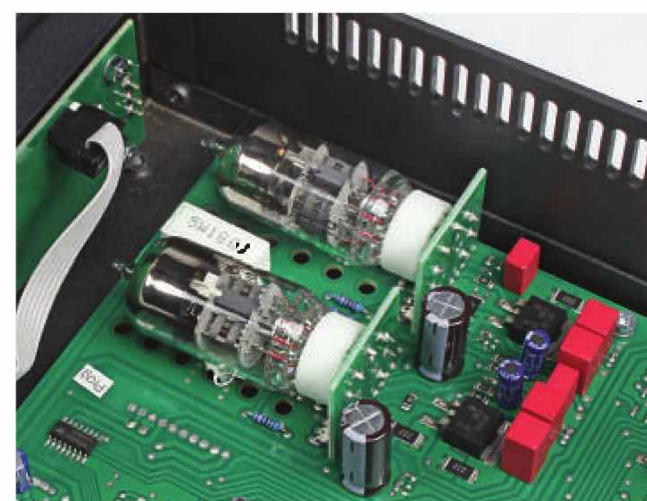
Here's what gives the DAC Box RS its 'valve sound' – a pair of Russian-made Electro-Harmonix 6922 double-triodes.
