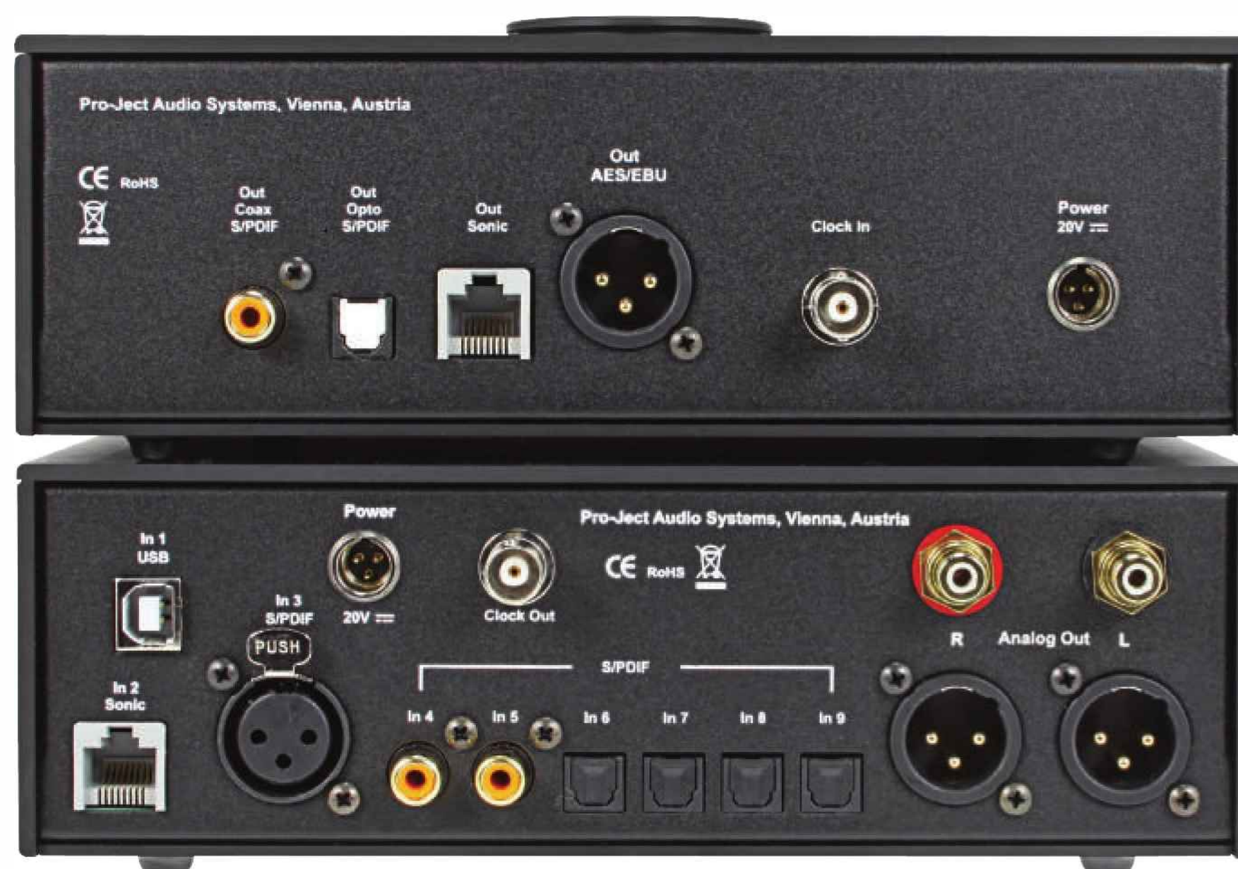
Plenty of connectivity - including the DAC's provision for USB, AES-EBU and six consumer-standard digital sources. On top of this is Pro-Ject's proprietary link, with separate cabling for clock and digital audio.
