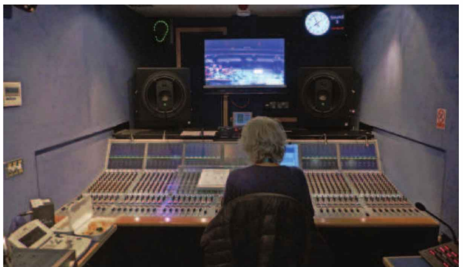
Within the confines of the OB truck, the engineer mixes all of the incoming signals on a Stagetec Nexus digital console for Radio 3.
