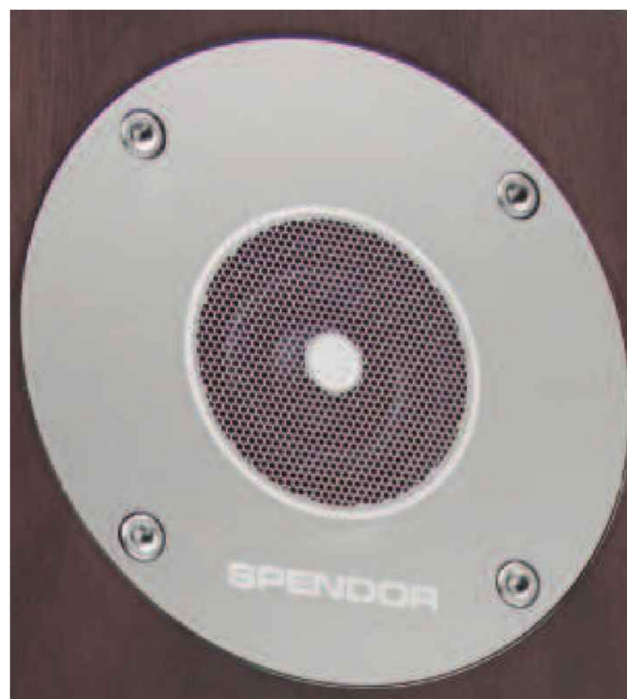
Spendor's new Linear Pressure Zone tweeter uses a steel mesh cover with a fabric foil to equalise pressure on each side of the diaphragm, giving a more linear response.
