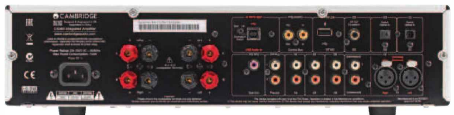
On the rear of the CXA80 twin speaker outputs are joined by a full set of analogue and digital inputs.
