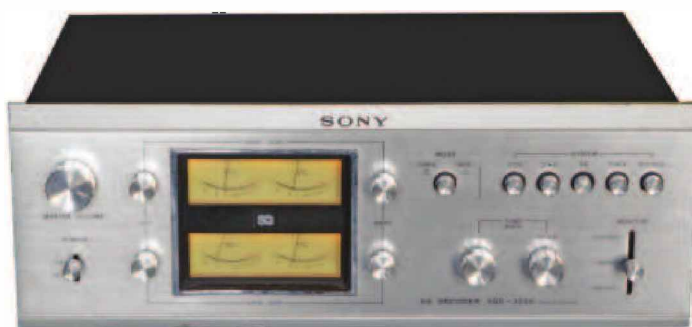
The 1973-vintage SQD-2020, which incorporated front-back and 'wave-matching' logic techniques to improve separation, was Sony's top-of-the-line 'add-on' SQ decoder for UK sale.
