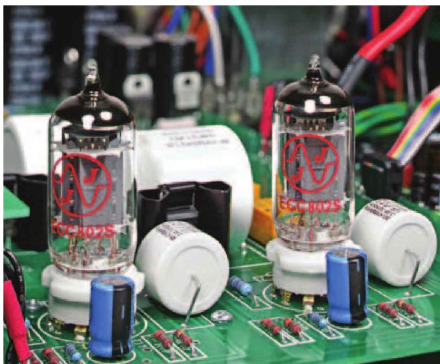
A pair of 12AU7 (ECC802) valves are used in the Pharaoh's input stage which in turn is coupled to Hypex UCD400 Class D output modules.
