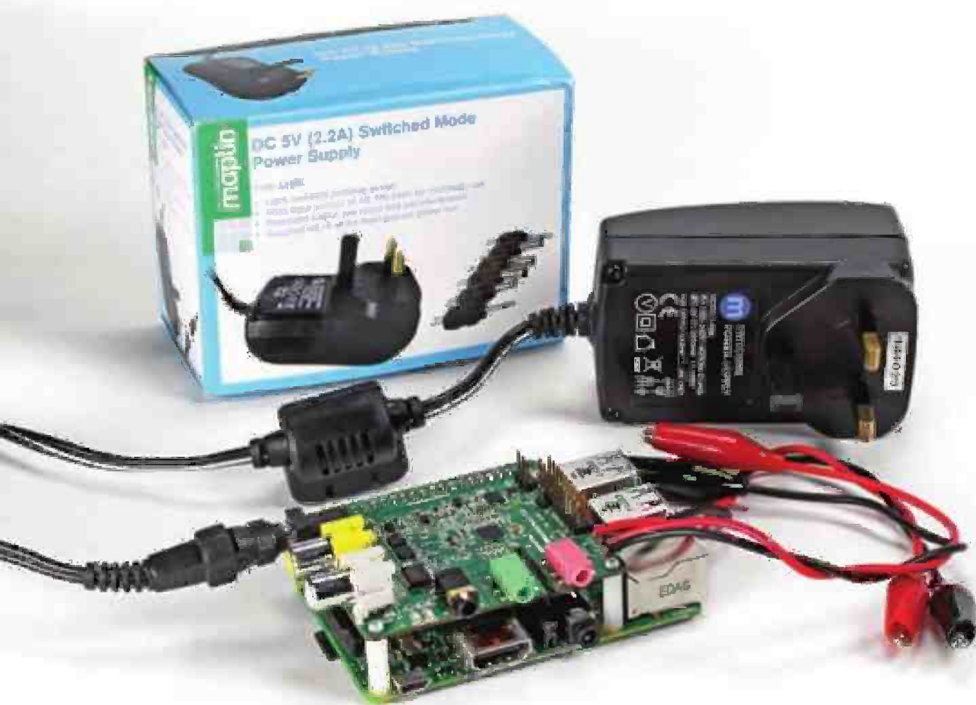
The Cirrus Logic audio board with loudspeaker leads soldered in and a suitable Maplins 5V, 2A smoothed power supply connected.
