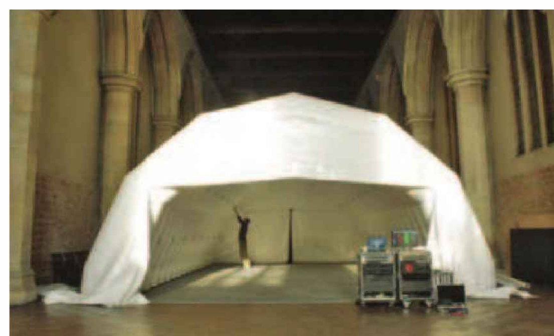
The construction is built as a series of ribs along its length with six speakers per rib.
