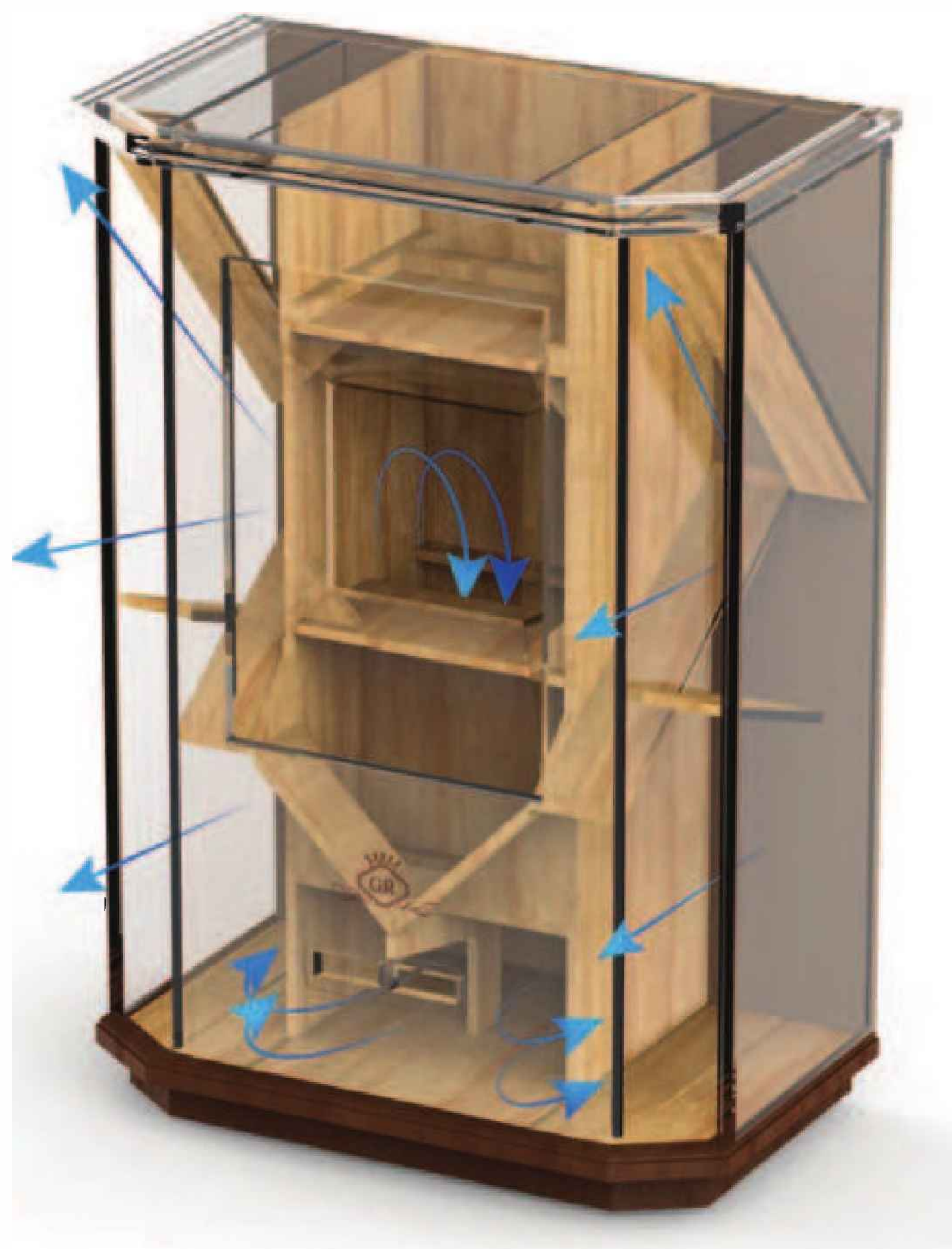
The complex internal cabinetry that forms a bass horn behind the huge 15in bass cone of Tannoy's 15in Dual-Concentric drive unit. The horn mouth is split into left and right, forward-firing side ports, hidden behind fabric grilles.
