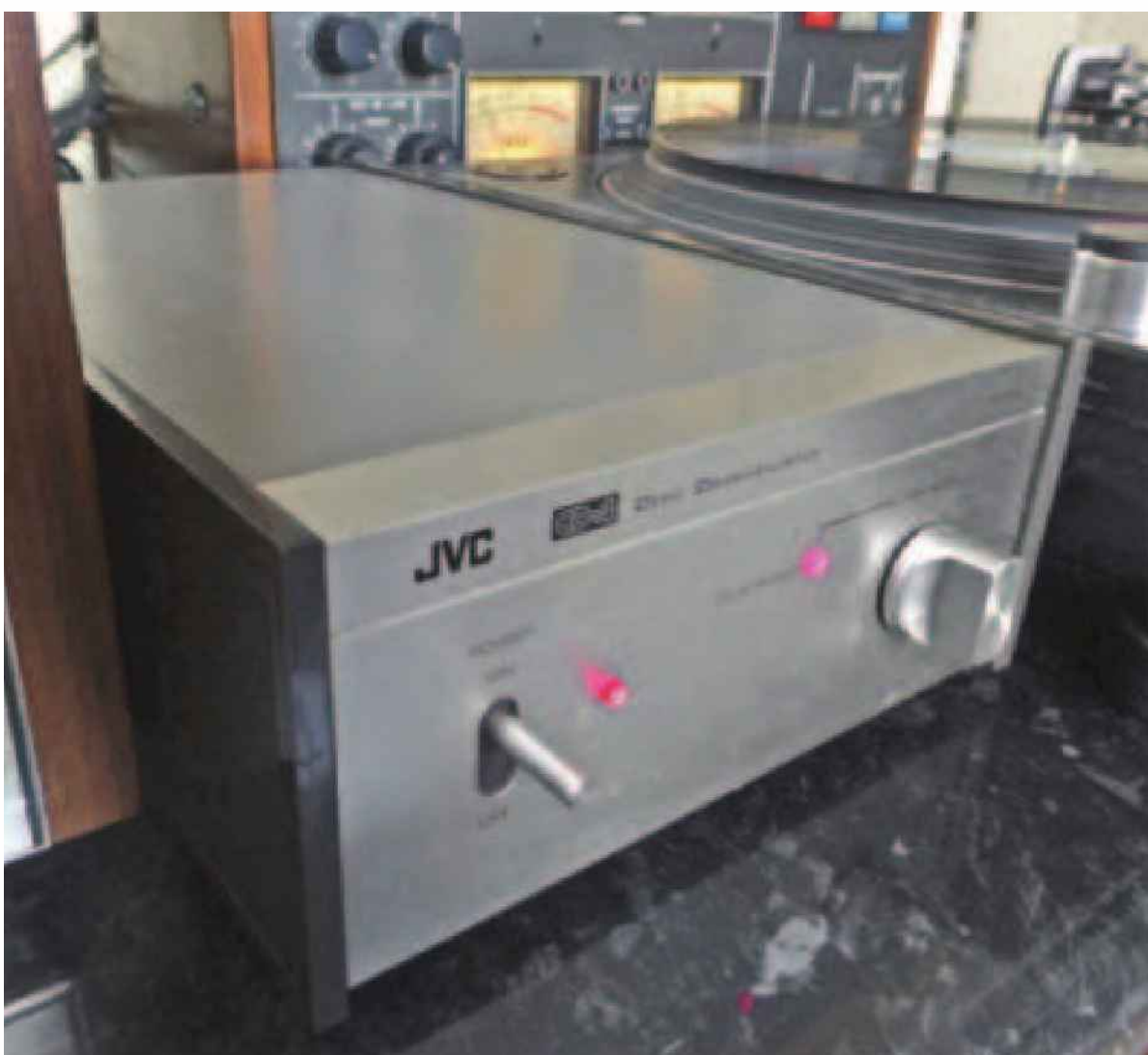
A device such as JVC's popular 4DD5 demodulator was needed to extract the quadrasonic information from the CD-4 discs.
