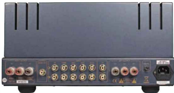
The DiaLogue Premium's rear panel features five line-level inputs as well as 8 Ohm and 4 Ohm 'speaker taps.
