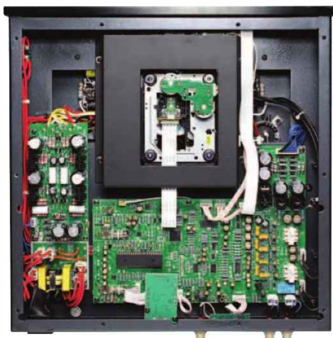
Inside the PrimaLuna Prologue CD player, with sliding drawer CD loading mechanism at top.
