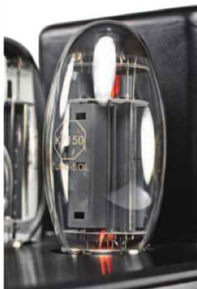
The new Tung-Sol KT150 is a power tetrode fitted with large power-dissipating anodes.
