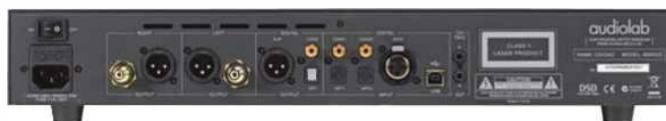
The rear panel carries balanced (XLR) and unbalanced (phono) analogue outputs, a balanced AES/EBU S/PDIF digital input, as well as electrical and optical S/PDIF digital inputs.
