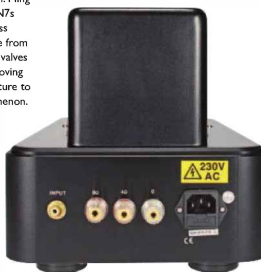
The rear panel has 8 and 4 Ohm outputs, as well as a power socket and analogue input.
