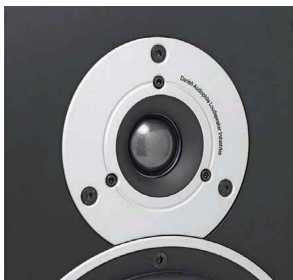
The 25mm soft dome tweeter has a shallow wave guide to aid dispersion.
