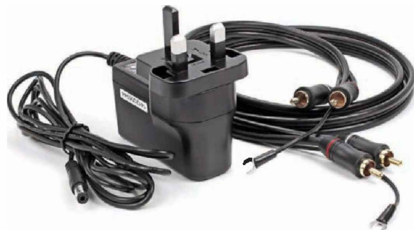
A wall-wart power supply provides 15V d.c. via a thin cable, so there is no hum producing a.c. anywhere near the hum sensitive cartridge and phono stage. An analogue signal cable is supplied, but not a digital optical cable. The earth must be connected, because there is no mains earth.
