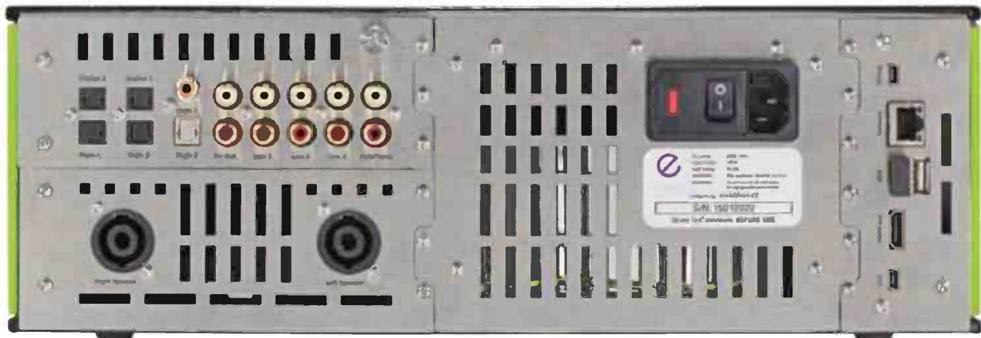
A full complement of digital and analogue inputs on the rear panel are joined, unusually, by a pair of Neutrik-style loudspeaker connections.
