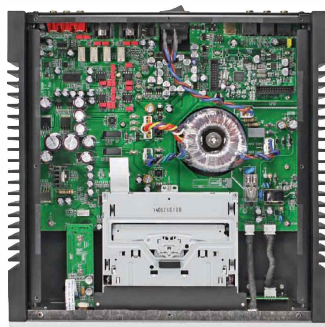
Internal appearance of the Artera Play is as neat as that of the exterior. Note the use of a linear power supply built around a toroidal-core transformer. High quality op-amps and capacitors are used in the audio stages.
