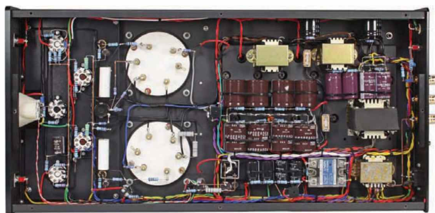
Another five transformers/chokes lurk underneath, plus hard wired audiophile components.
