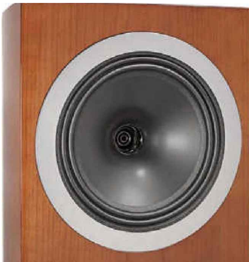
The horn loaded tweeter, with pep-perpot waveguide, fires out through the centre of the bass/midrange cone.
