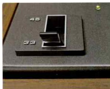
*The speed control is coupled, via a system of levers underneath the deckplate, to a pair of fingers that push the belt up or down and onto the relevant pulley step. Effective – and very easy to use.*
