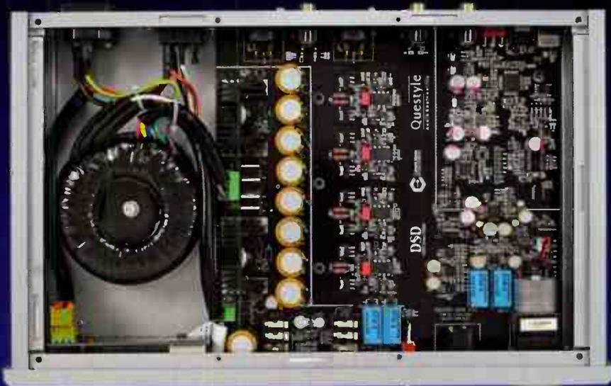
*A busy but well laid-out interior, with the (linear) power supply selection on the left. The middle section is occupied by the CMA output amplifiers, while the DAC circuitry can be seen on the right. High-quality components are in evidence, but on close inspection some circuit-board bodes are evident.*
