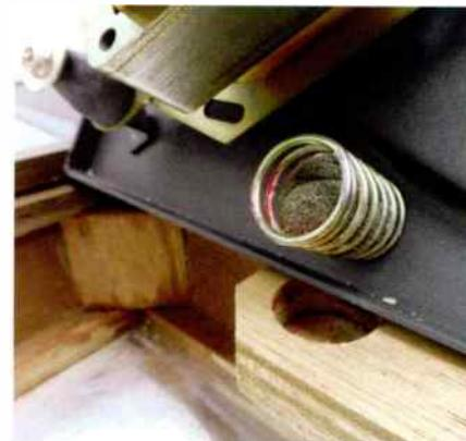
**The PL-12D's simple spring suspension system. The foam within provides a modicum of damping but may need replacing if deteriorated.**
