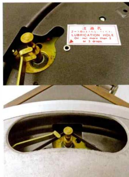
*The PL12D has a 'classic' stepped motor pulley to effect speed change. You don't have to fumble with the belt yourself. Here, a 'fork' coupled to a control lever shifts the belt onto the appropriate pulley. You can also see a lubrication hole for the motor, a four-pole synchronous design.*
