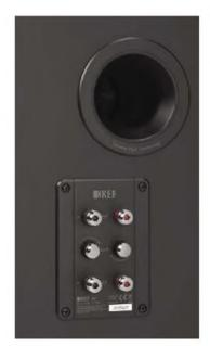
The connection panel carries bass and mid/treble inputs for bi-wiring, but they are connected by a simple screw switch for mono-wiring.
