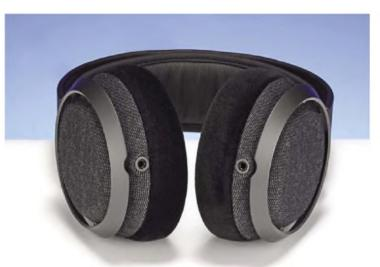
Each earpiece has its own 3.5mm three-pole (stereo) input jack socket. An unusual choice: this is usually a mono (two pole) socket. But the stereo jack is more widely available, making a balanced or specialist cable easier to construct or purchase.
