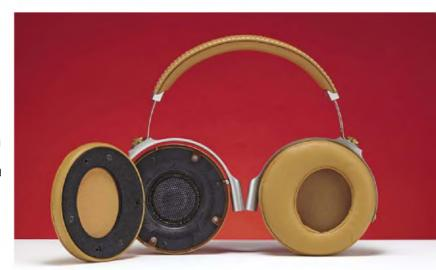
The ear pads attach by magnets and can be simply removed to reveal the drive units, as at left. Each cradle carries a 3.5mm mono output jack, seen at centre, to provide optional balanced operation.
