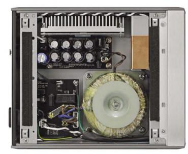
The linear power supply carries a large toroidal mains transformer, banks of smoothing capacitors and even a heatsink for what likely is a high current voltage regulator.
