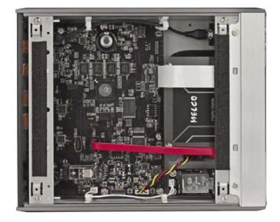
Internally, the N10 carries a circuit board packed with Surface Mount Devices (SMD). Its 3TB hard disc drive (HDD) can be seen at right.
