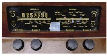
Four knobs cover tone/power off, volume, wavechange/gram selection and tuning. The backlit side-by-side tuning scales are marked with stations. Right covers medium-wave, left covers VHF-FM and long-wave.
