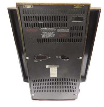
Hardboard backs, with cooling slots through which the reassuring glow of valves can be seen, were common practice in radio construction since the 1930s.
