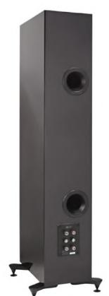
Upper and lower reflex ports tune the internal bass chambers slightly differently, to smooth low bass and give an even amplifier load.
