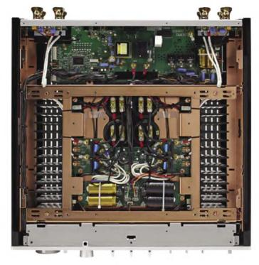
A rigid steel chassis copper plated to reduce eddy currents is made obvious in this underside view. At left and right sit heatsinks below vents, but the amplifier ran cool in normal use.
