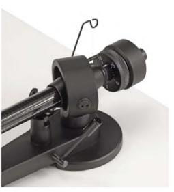
The arm has a damped cue platform with lever, a calibrated rear counterweight and simple weight-end-thread bias that passes over a wire support. a small external wall-wart power supply unit, switch-mode of course. This means the turntable is not mains earth connected, point being the possibility of hum from an earth loop is eliminated. There are no high voltages in the turntable either: put it in a tub of water and you won't get a shock – to illustrate a point!
