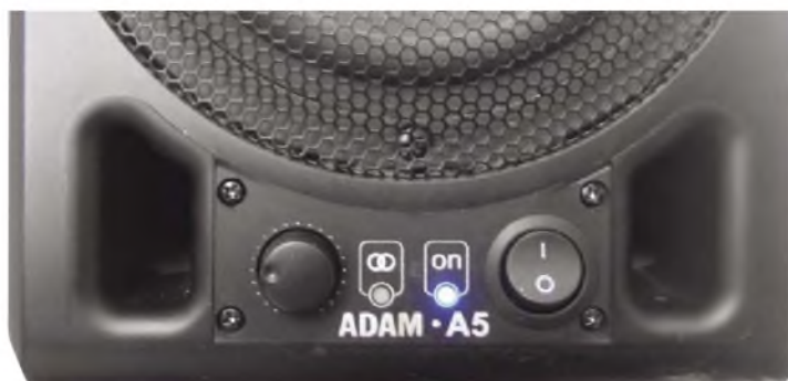
Just beneath the woofer are the volume control and that trouble-prone mains switch. In addition to a power-on LED is one that illuminates when the 'stereo link' mode is active.
