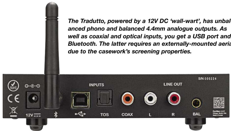
**The Tradutto, powered by a 12V DC 'wall-wart', has unbalanced phono and balanced 4.4mm analogue outputs. As well as coaxial and optical inputs, you get a USB port and Bluetooth. The latter requires an externally-mounted aerial, due to the casework's screening properties.**
