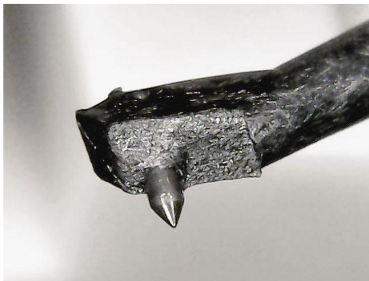
**This picture shows the fibrous nature of the cantilever and what appears to be a ground-on flat to accept the stylus shank.**
