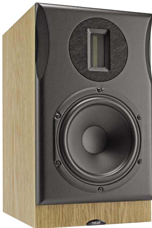
**The Majistra is solidly built and heavy, made so by an internal isobaric chamber carrying a second 170mm bass unit. At top, the ribbon tweeter, with soft surround to absorb surface waves.**
