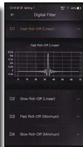
**Settings available in the Mango player app with (at right) the list of seven digital filters together with a time domain graph of impulse behaviour.**
