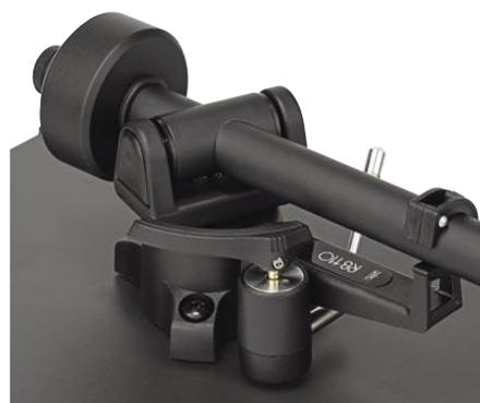
**The rear counterweight has no weight calibration dial, making stylus scales essential. Rega set VTF at 2gms but Audio Technica recommend 2.5gm minimum.**
