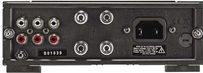
**At rear the small io amplifier has just three phono socket inputs, two for Line and one (left) for a turntable. The two pin IEC mains input shows it is not earthed, allowable in IEC Standards if certain safety conditions are met.**
