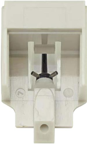
**Inside the removable stylus assembly lie a pair of cylindrical magnets attached to the cantilever, ahead of the hinge. This is Audio Technica's V magnet arrangement.**
