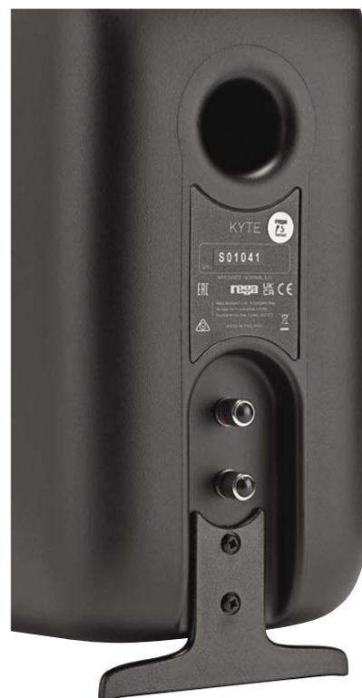
**At rear of the Kyte loudspeakers a plastic stabilising bracket keeps the curved cabinets stable. With a single pair of terminals bi-wiring is not possible At top a port tuned to 60Hz measurement showed.**
