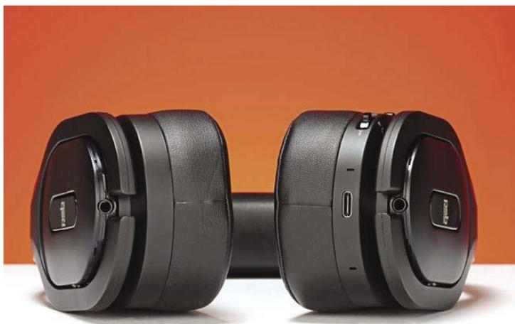
**Unusually, PSB has fitted a 3.5mm socket to each earcup. If you're using a 'wired' device, you no longer have to worry quite so much about where it's positioned. There is however only one USB-C socket, which is needed to charge the M4U 8 MK2 for of up to 25 hours of continuous use.**
