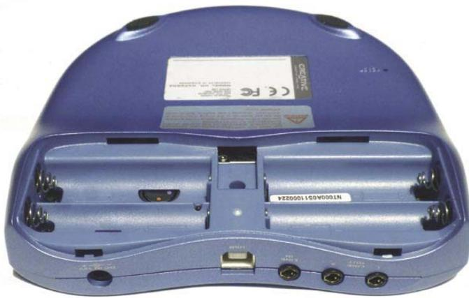
**Only four hours of continuous listening was possible on a full charge of the supplied NiMH cells, which live under a tricky-to-detach cover. Thankfully, the unit could also be powered from an external 12V DC supply – such as a car cigarette-lighter cable, or the supplied mains unit.**
