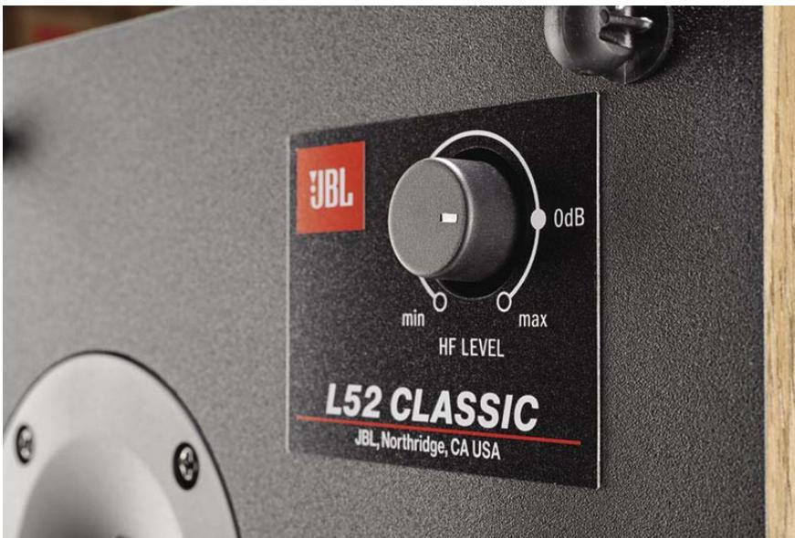
**A unique feature of the L52 Classic is adjustable tweeter level. Set to 0dB the 'speaker measured flat. A few dBs of treble lift are possible, or a large range of treble cut.**
