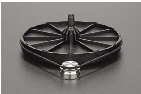
**Belt drive to a central hub of moulded Phenolic. To change speed (33rpm / 45rpm) the platter must be removed at the belt moved to a different pulley groove. It's set at 33rpm here.**
