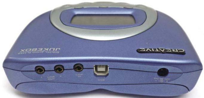
**DSP wizardry inside the DAP Jukebox facilitated surround decoding, the two stereo line outputs feeding front and rear channels to external amplification. Equally-unusual is the line input, which allowed the unit to be used as a CD-quality hard-disk recorder.**
