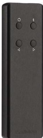
**Earmen has built the simple remote - which duplicates the front panel's source selection, Bluetooth and standby buttons - into a solid aluminium case.**
