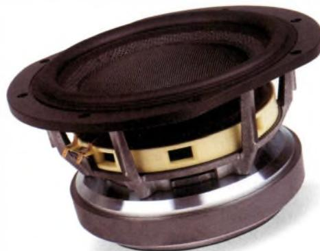
► wave absorption through a sculpted, tapered line. The midrange driver continues B&W's woven Kevlar cone tradition, and has undergone further development in the fine-tuning of the edge termination of the cone for improved energy decay properties. In addition, the driver itself is gel-decoupled from the head enclosure. The tweeter is further decoupled from the mid unit at a very low frequency (around 10Hz) this pioneered by Naim and Roksan, via an anti-vibration mount.
