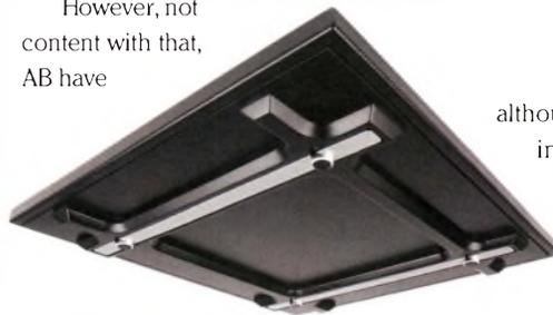
developed a superior platform, the StrataBASE 2. The same size as a BASE 02, this employs two slabs of MDF arranged as a constrained layer, with additional lateral as well as longitudinal bracing on the underside. It's heavier (visually and physically), more expensive but it's also far more effective.
