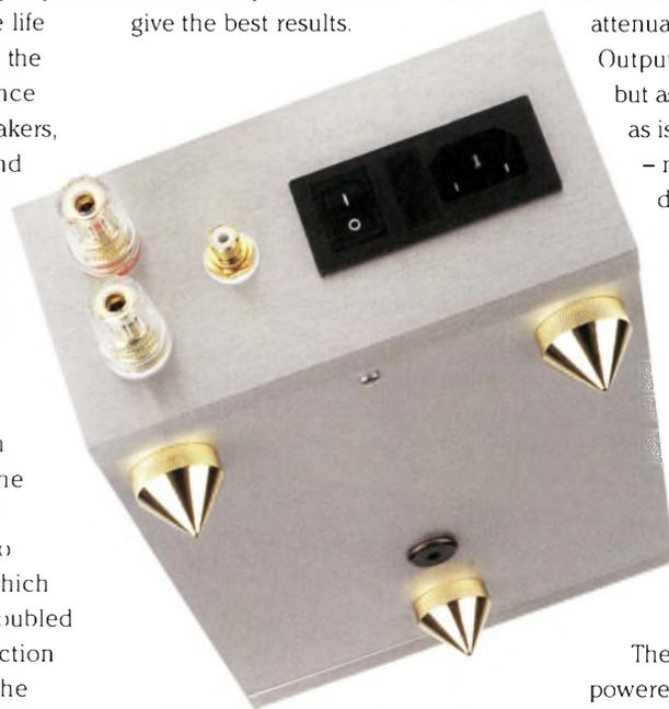
The transformer approach is designed to offer a more flexible volume control that will work with a wide range of components and cables. They are not perfect of course and the TX-102 does run into bandwidth limitations at the point where it is offering the least attenuation. Ordinarily however, if your source has an output impedance of 1 kOhm or less, the transformers will provide a bandwidth of 10Hz – 10kHz.
