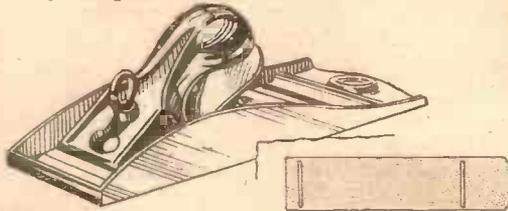
A "Bullnosed" plane is made of metal with the blade controlled by an oval eyed screw. The smaller illustration is a view of the underside of the plane, showing the two alternative slots. Remember that a plane should never be stood flat on a bench or the blade is likely to get scratched or indented.
