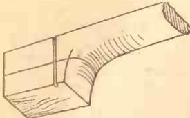
Fig. 3.—The shoulder block beneath the inner end of the neck, with a groove for the plywood body.
