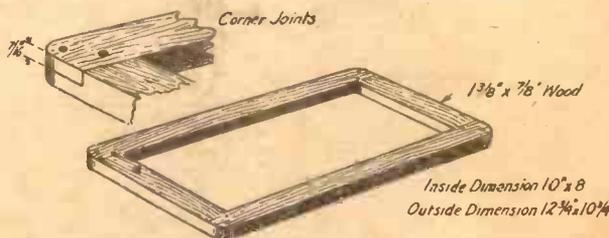
Fig. 3.—The chase in which the type is held or set.
