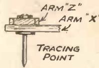
Fig. 4.—How the tracing point is made.
