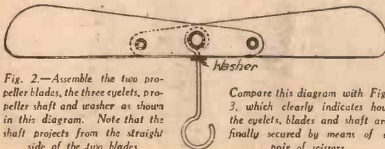
Fig. 2.—Assemble the two propeller blades, the three eyelets, propeller shaft and washer as shown in this diagram. Note that the shaft projects from the straight side of the two blades.
