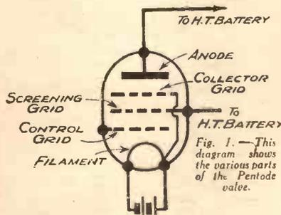
Fig. 1.—This diagram shows the various parts of the Pentode valve.
