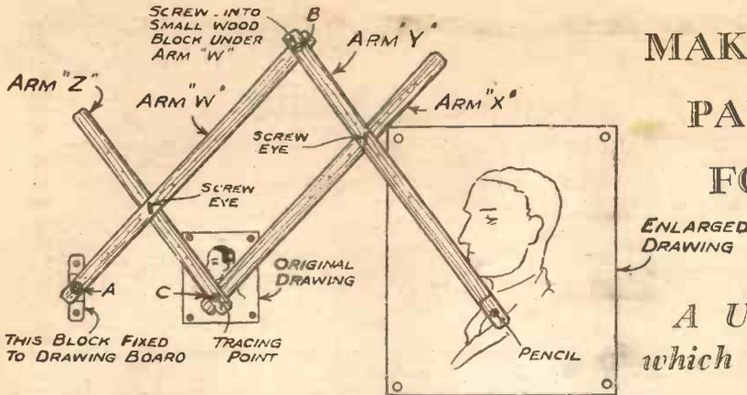
Fig. 1.—The pantagraph completed. The assembling of the parts is shown in this diagram.
