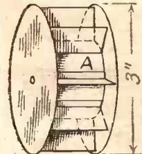
Fig. 5. Assemble the sand-wheel in the manner shown here.
