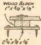
Fig. 3.—The block for clamping the pantagraph to the drawing board.
