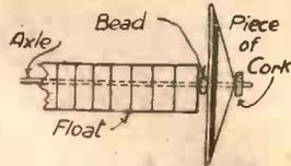
Fig. 6.—How to fix axle and wheels.
