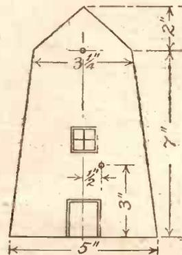
Fig. 4. How to mark out the mill-house.
