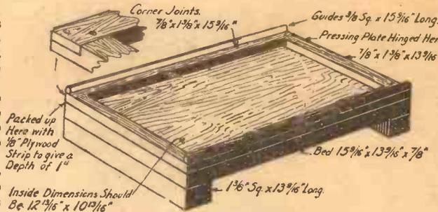
Fig. 1.—How to make the press bed.
