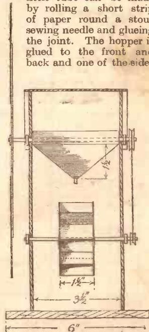
Fig. 3. The hopper and sand-wheel mechanism.
