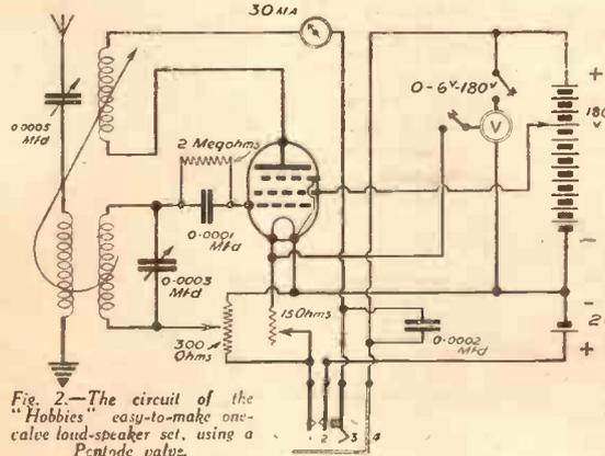
Fig. 2.—The circuit of the “Hobbies” easy-to-make one-valve loud-speaker set, using a Pentode valve.
