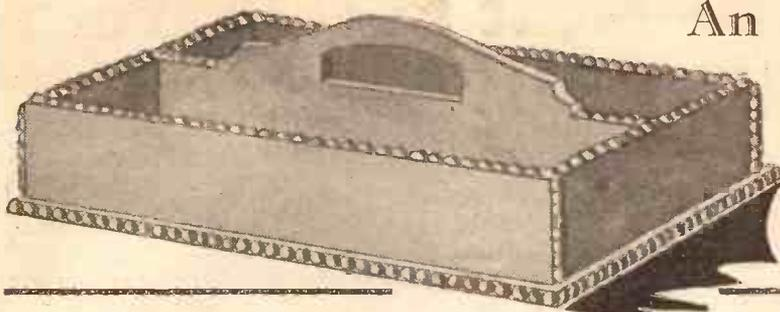
THE illustration above shows an ornamental but easily-made knife box, which will come well within the scope of the amateur woodworker, as the parts only need to be cut from fretwood, glued and nailed together, and ornamented with fancy beading.
