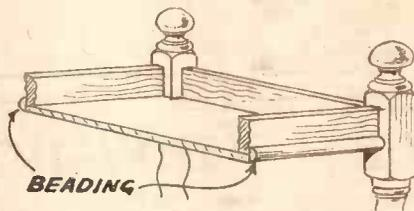
Fig. 4. The top tray and rails broken to illustrate construction and particularly the way in which the half-round beading covers the join of the tray to the rail.
