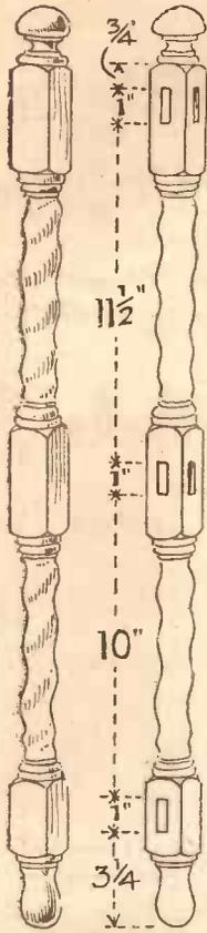
Fig. 1. On the left is the leg as bought and on the right measurements for cutting the necessary mortises.
