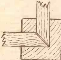
Fig. 2. A section through the leg joint showing how the two chamfered rails meet inside the mortises at the corner.
