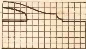
Fig. 2.—The squares represent  $\frac{1}{4}$  in. spaces, so you can draw the proper shape on to the wood.
