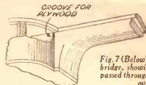
Fig. 7 (Below)—The lower bridge, showing the strings passed through and brought over.
