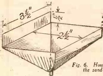
Fig. 6. How to assemble the sand-hopper.
