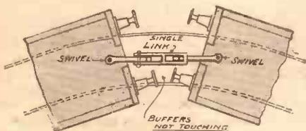
Fig. 2. Buffer locking on sharp curves.
