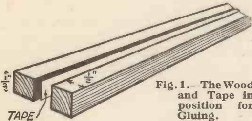
Fig. 1.—The Wood and Tape in position for Gluing.
