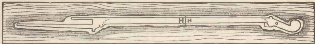
Fig. 1.—The Pattern of the two parts of the Neck are pasted on the wood like this, to make one complete Length.
