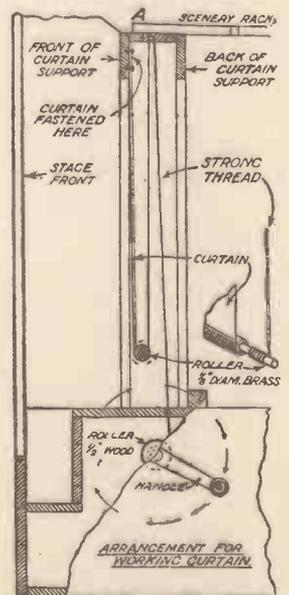
This Diagram explains how to work the Drop Curtain.
