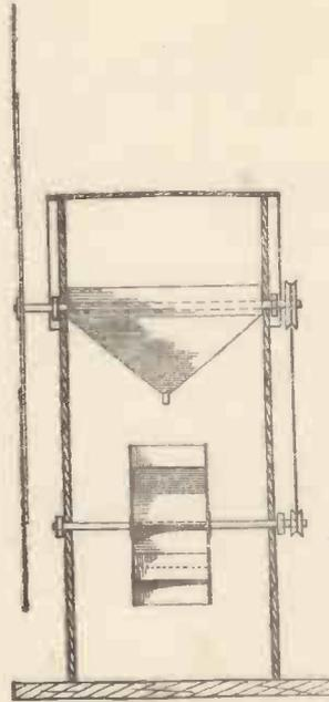
The Hopper and Sand-wheel Mechanism.
