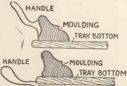
Fig. 3.—The manner of fixing the Handles is shown above. One is to the Moulding, and the other is under the Tray.
