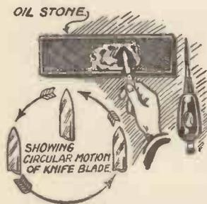
Diagram showing how to sharpen a pocket-knife blade on an oil-stone.
