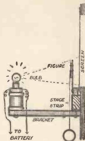
Fig. 5. —The Lighting Arrangement.
