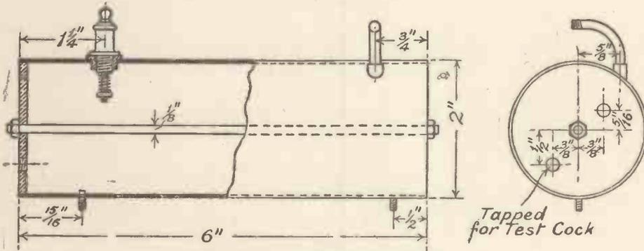
Fig. 3.—How the Boiler is made.
