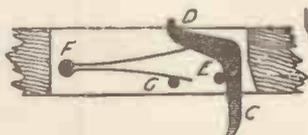
Fig. 4.—The Trigger for releasing the Bolt.
