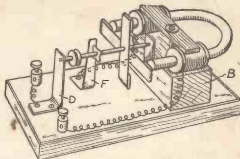
Fig. 1.—The Complete Electric Motor.
