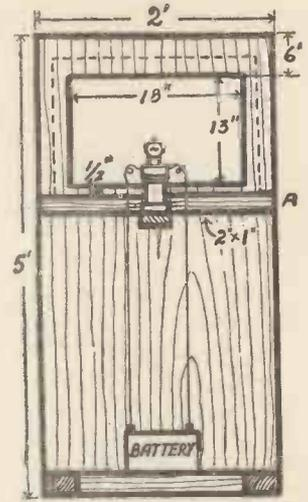
Fig. 3.—The Measurements for cutting the Stage Opening.
