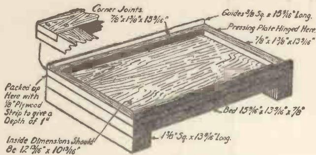
Fig. 1.—How to make the Press Bed.
