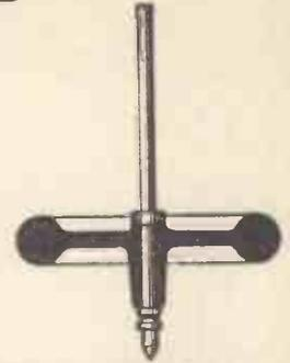
Fig. 2.—The Body of the Top can be made from a single Brass Casting.
