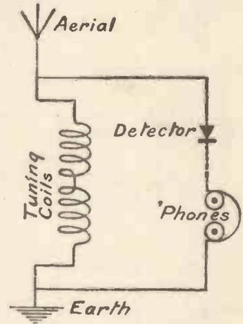
Fig. 3.—The Circuit diagram.
