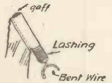
Fig. 2.—The "Gaff" is secured as shown.
