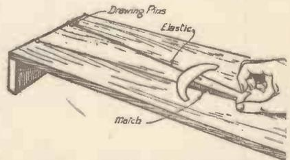
Fig. 6.—How to arrange the Catapult.
