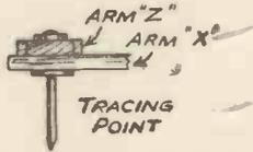
Fig. 4.—How the Tracing Point is made.
