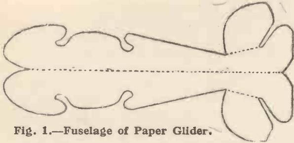
Fig. 1.—Fuselage of Paper Glider.
