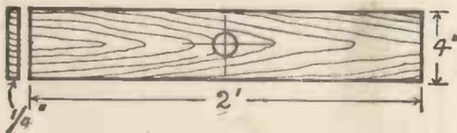
Fig. 2.—The Measurements of the Wood for the Frame Aerial.
