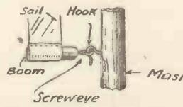
Fig. 3.—How the Boom is secured.
