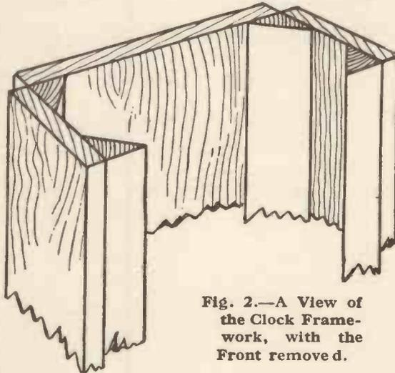
Fig. 2.—A View of the Clock Framework, with the Front removed.
