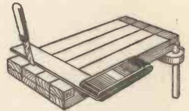
Fig. 4.—Setting out Rails for "Barefaced" Tenons.
