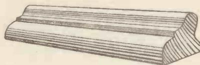
Fig. 1.—This is the Moulded Edge you buy in Strips to form the Tray Sides.
