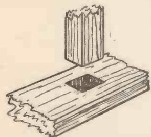
Fig. 1.—The Base with hole cut to take the upright.
