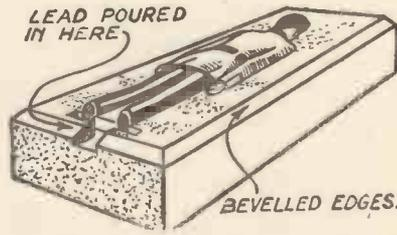
Fig. 2.—Taking an impression of a toy stationmaster in the plaster Mould.
