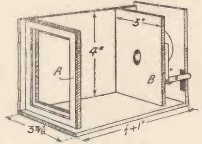
Fig. 2. — Details for fixing the Lens Board.
