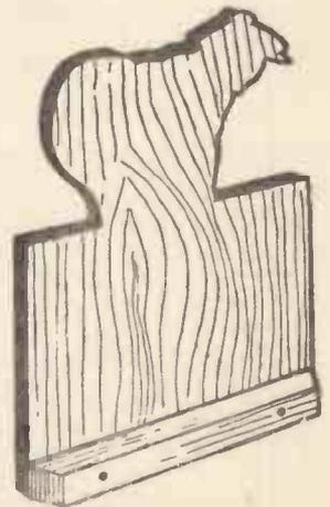
Here the Base is merely a strip of wood glued and nailed along the back.
