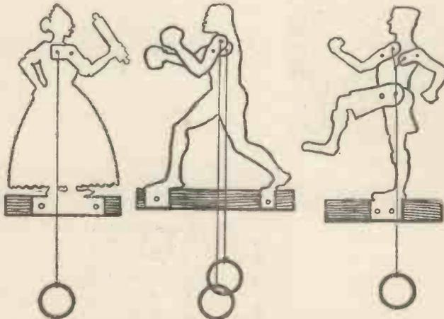
Fig. 4.—Details for making the Figures.
