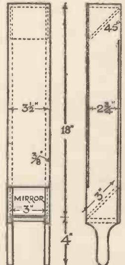
This diagram shows how to assemble the various Parts.
