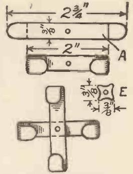
Fig. 4.—How to make the Armature.
