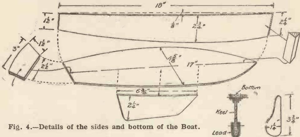
Fig. 4.—Details of the sides and bottom of the Boat.
