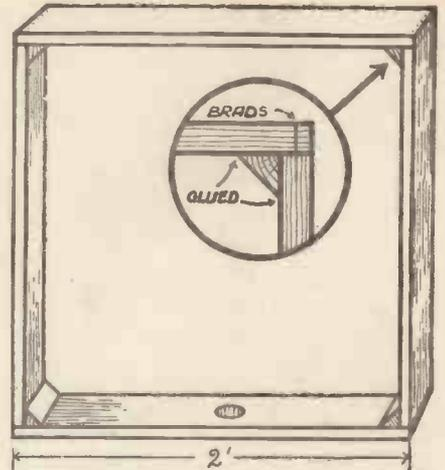
Fig. 3.—How the Frame Aerial is assembled. Inset gives details of the Corner Joints.
