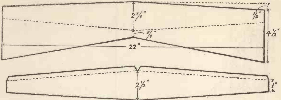
Figs. 3 and 4.—Details of the Wings.
