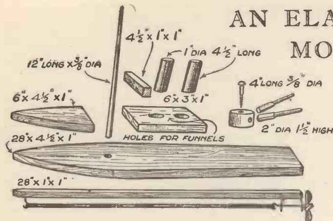
Fig. 2.—The Component Parts of the Battleship.
