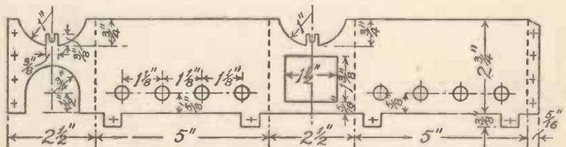
Fig. 4.—How to mark out the Firebox.
