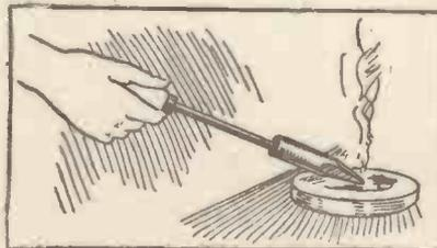
How to tin the Soldering Iron.
