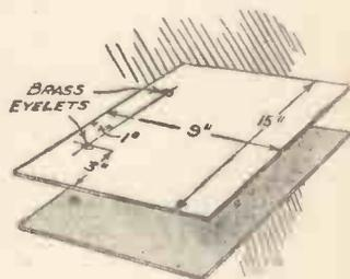
Fig. 7.—How to make the Cover.
