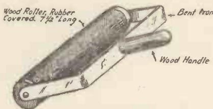
Fig. 6.—Roller for Inking the Type.
