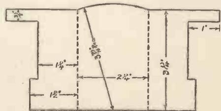
Fig. 10.—The Sides and Back of the Cab.
