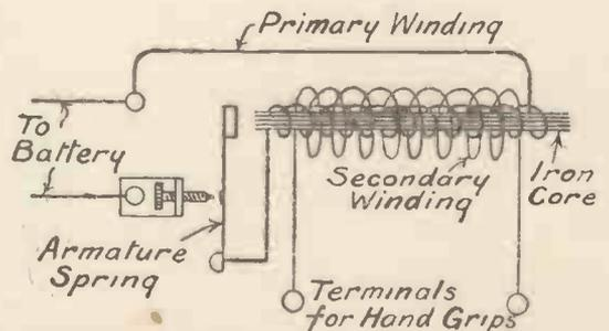
Fig. 4.—The Coil should be Tested by connecting up to a Dry Cell.
