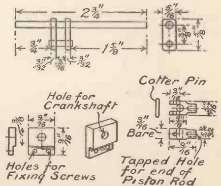
Fig. 8.—Details of Crankshaft, Bearings, and Piston Rod Head.
