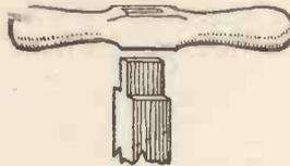
Fig. 4. — How to fix the Handle.
