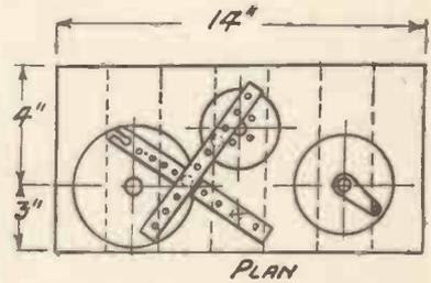
Fig. 3.—The position of the Pulleys.
