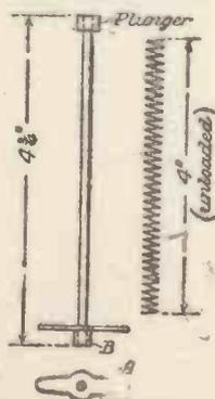
Fig. 3.—Spring-rod, Catch-plate, and Spring.
