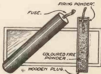
Fig. 3.—Details of the Container for holding the Coloured Fire.
