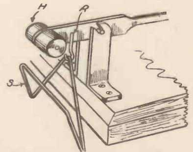
Fig. 5.—How the Letter-Holder is made.
