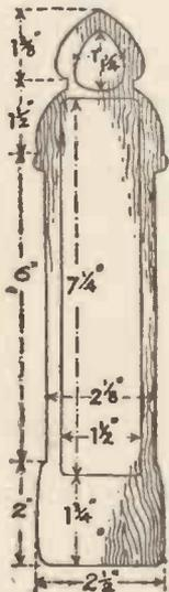
Fig. 1.—The measurements of the Pencil-Box.
