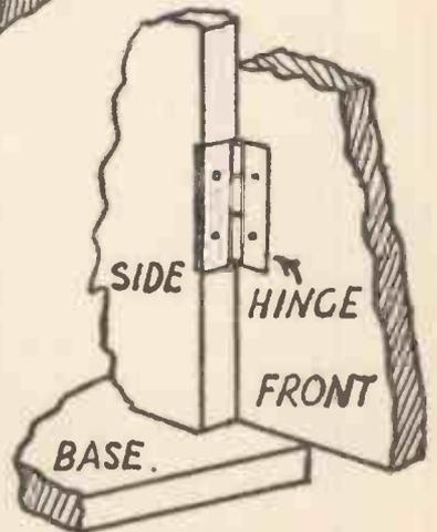
Fig. 5.—The way the Hinged Front is Fitted on.
