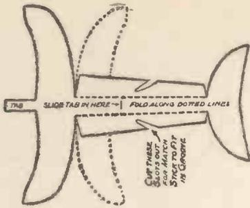
Fig. 5.—How to make a simple Catapult Glider.
