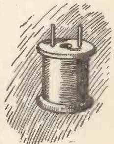
Two nails with their heads filed off are driven in to a cotton reel as shown.
