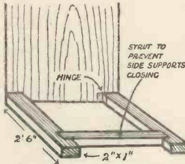
Fig. 2.—The Supports for the Front.
