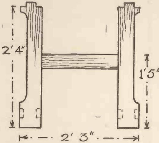
Fig. 2.—An Elevation of the Chair front.
