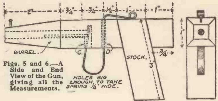
Figs. 5 and 6.—A Side and End View of the Gun, giving all the Measurements.
