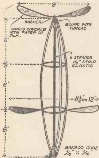
Fig. 3.—The Completed Model Helicopter.
