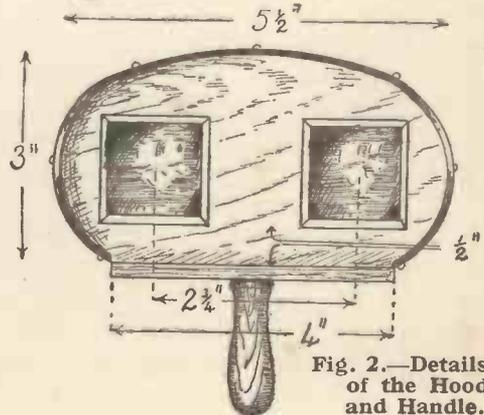
Fig. 2.—Details of the Hood and Handle.
