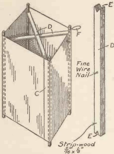
The completed Box Kite and (right) the Diagonal Stretchers.
