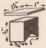
Fig. 7.—How to make the Stacks for the Chimneys.
