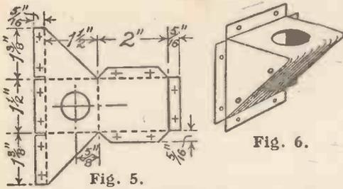
Figs. 5 and 6.—How to mark out and assemble the Chimney Support.
