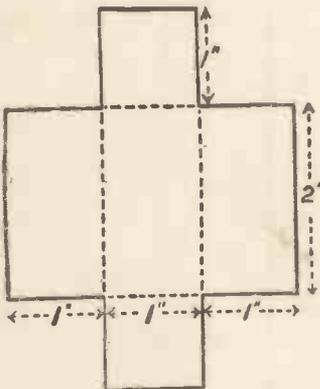
Fig. 1.—How to make the Mould.
