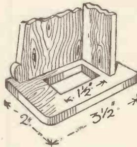
Fig. 2.—Details of the Floor.
