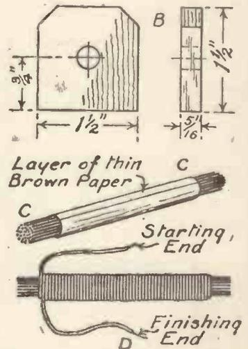
Fig. 2.—How to Wind the Coil.
