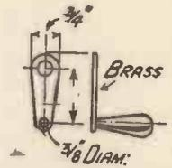
Fig. 9.—The Driving Pulley with Handle attached.
