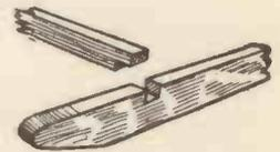
Fig. 13.—How to Joint the Frame.
