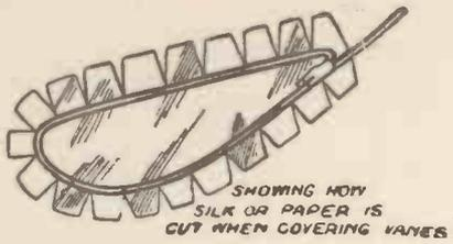
Fig. 5.—How to cover the Wire Propeller.
