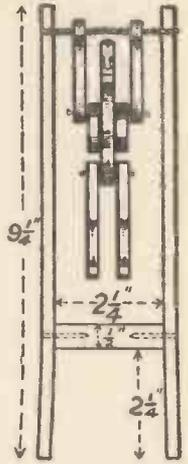
Fig. 2.—The Frame Measurements.
