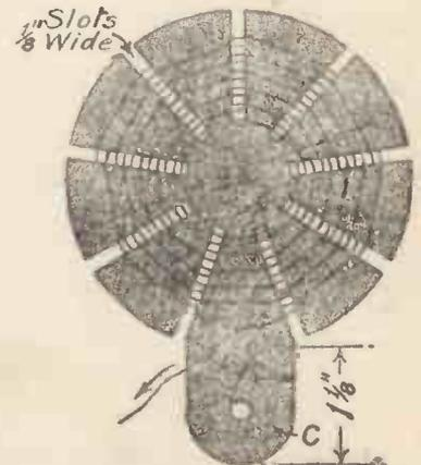
Fig. 2.—How the Basket Coils are made.
