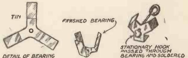
Fig. 1.—Details of the End Bearings.
