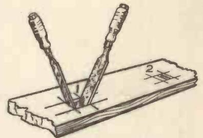
Fig. 8.—How to cut the Mortise.
