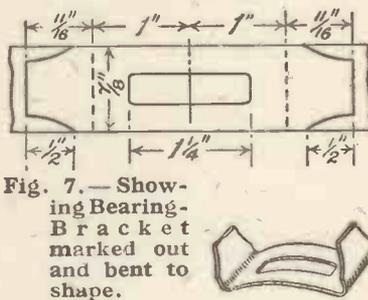
Fig. 7.—Showing Bearing Bracket marked out and bent to shape.
