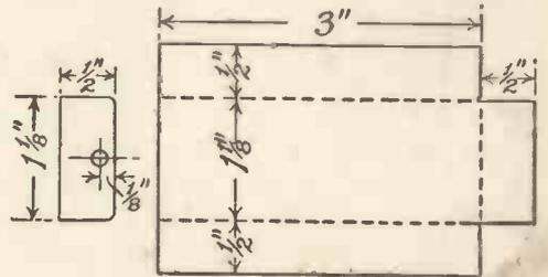
Fig. 10.—Tinplate Blank for forming Drip Tray of Lamp.
