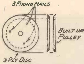
Fig. 5.—Details of the Pulleys.
