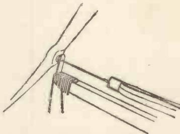
Fig. 4.—Details of the Bearing, and Propeller Shaft.
