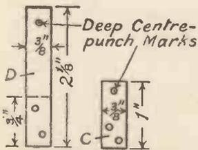
Fig. 5.—The Bearing Supports.
