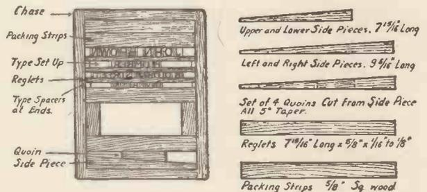
Fig. 4.—How the Type is Set in the Forme.
