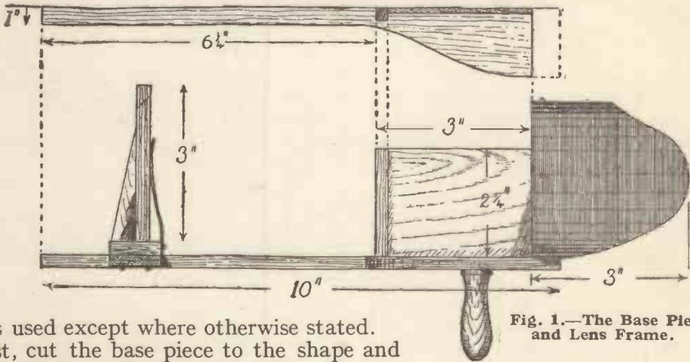
Fig. 1.—The Base Piece and Lens Frame.
