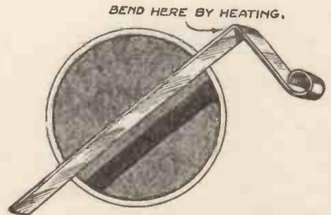
Fig. 7.—The Firing Spring.
