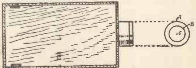
Fig. 7.—A sectional view of the Camera. A is the rim of a pill-box; B, tin-foil lens; and C, small pin-hole.
