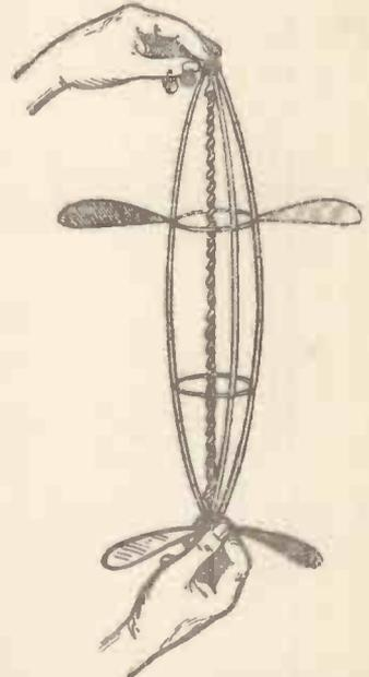
Fig. 8.—How to launch the Model Helicopter.
