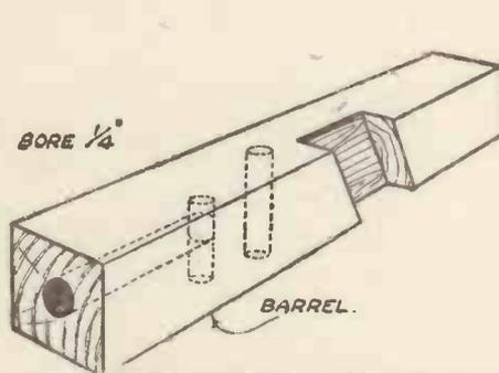
Fig. 1.—The Barrel should be Cut and Shaped as shown.
