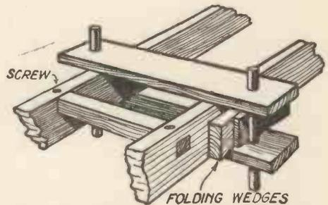
Fig. 12.—Showing position of Screw.
