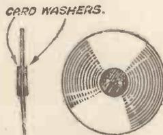
Fig. 5.—The Wheel with cardboard discs attached to strengthen it.
