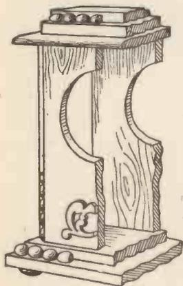
Fig. 1.—The Case broken through to show the General Construction.
