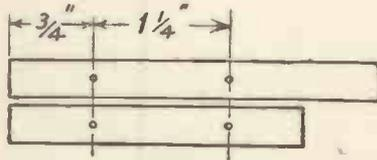
Fig. 2.—Method of Marking Supports for position of Spindles.
