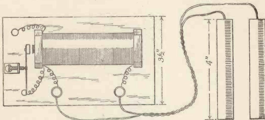
Fig. 1.—Plan View of the Shocking Coil.
