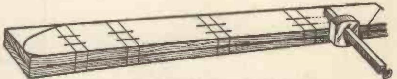
Fig. 7.—Marking out Sides for Cutting.
