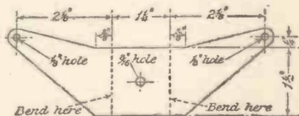
Fig. 6.—How to mark out the Cradle.
