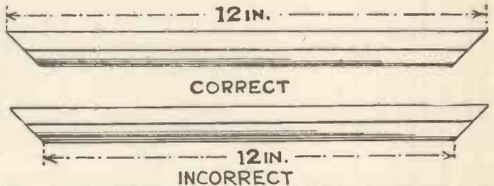
Fig. 2.—The Right and Wrong of Measuring Lengths of Moulding for the Edges.
