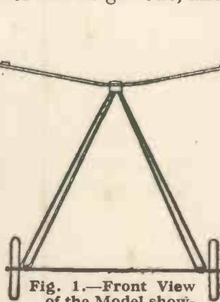
Fig. 1.—Front View of the Model showing the Dihedral Angle.
