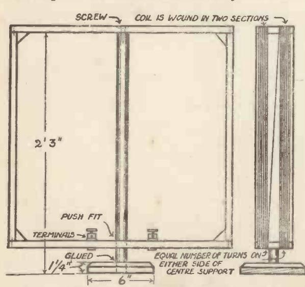
Fig. 4.—The whole Frame is supported by a length of Small-gauge Broom-handle.
