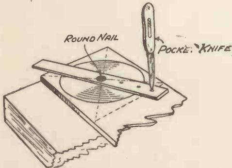
Fig. 4.—Cutting Discs from Plywood.
