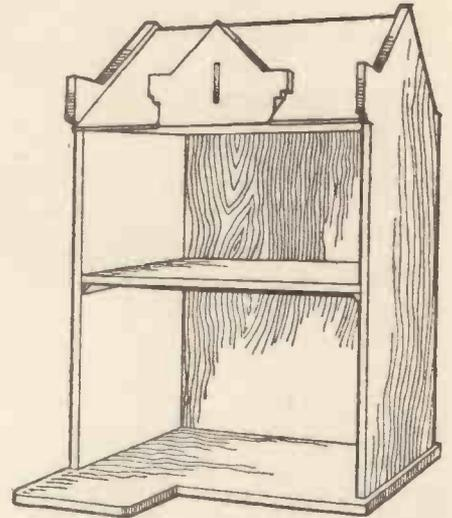
A Picture of the Skeleton Framework without the Door, to show the General Construction.
