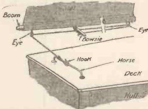
Fig. 1.—The Main Sail must swing from side to side to an extent governed by the cord called the Main Sheet.
