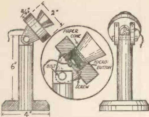
Fig. 5.—The Stand for the Microphone.
