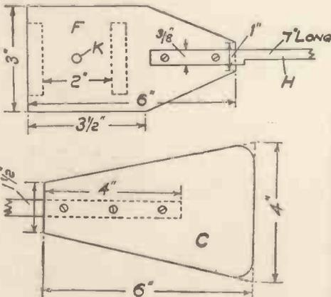
Fig. 3.—How to make the Sails and the Tailpiece.
