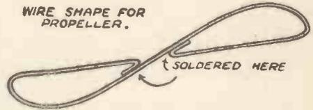
Fig. 6.—The Wire Propeller Frame.
