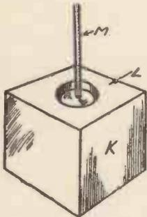
Fig. 4.—The Mould for the Counterpoise Weight.
