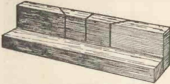
This is the Mitre Tool used to guide the Saw at the right angle in cutting the Strips.
