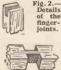
Fig. 2.—Details of the finger-joints.
