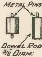
Fig. 7.—The Spindle Supports.
