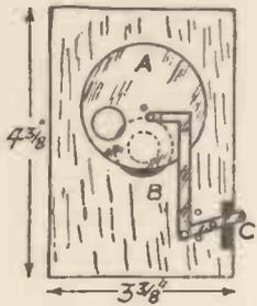
Fig. 4.—Method of fixing the Shutter.
