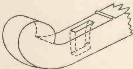
Fig. 3.—A Hole is cut downwards through the Neck to take the Key through the little Hole.
