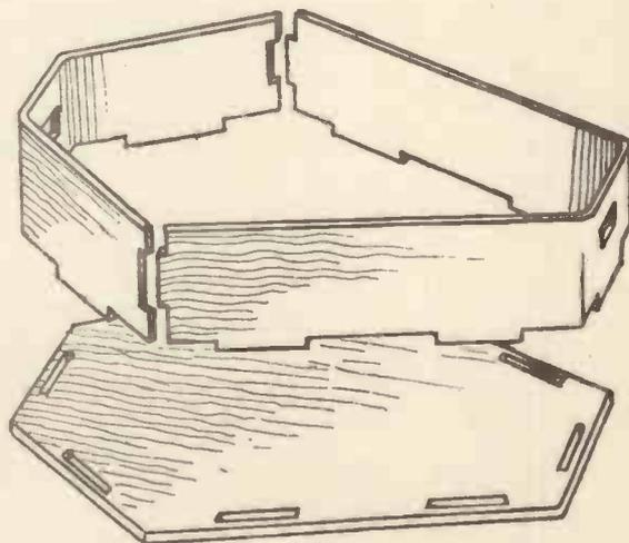
A General View of the Body work, with the two parts forming the Sides.
