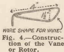
Fig. 4.—Construction of the Vane or Rotor.
