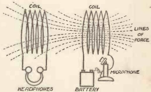
Fig. 1.—The Principle on which the Telephone works.
