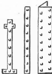
After painting with varnish, the strips should be cut to correct lengths, according to the height of the wagon sides to which they are to be fitted, and they should be folded neatly along
