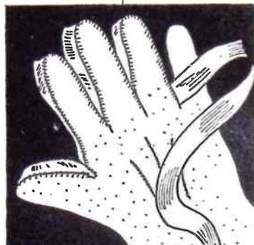
Simple method of joining seams—one continuous strip
