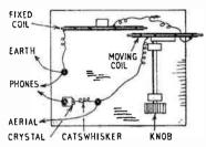
Fig. 3—Receiver connections
