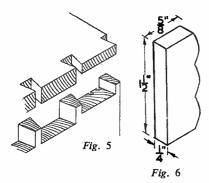
Prepare the four pieces to 8½ ins. wide and ½ in. thick, remembering that the appearance of the finished article depends very largely upon the accuracy with which the wood is prepared. Put the two ends in the vice together and
