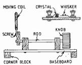
Fig. 2-Details of Detector and Tuning Control
