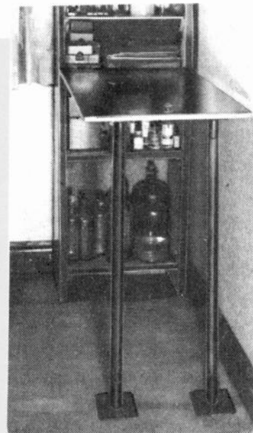
The door has been lifted and legs placed in position
