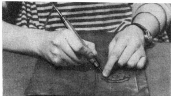
Fig. 2—Here the bent tracer is being used to impress an outline on the back of the sheeting.
