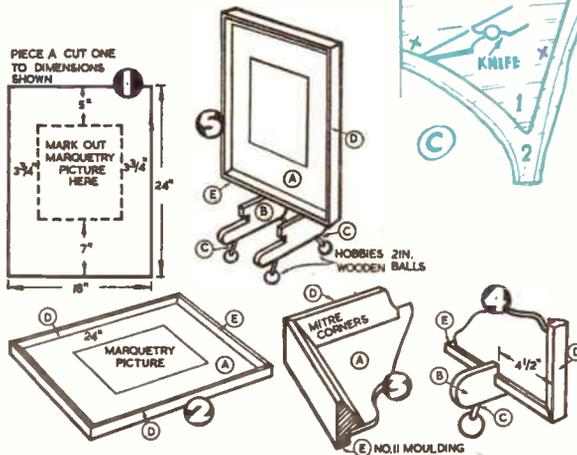
The addition of the feet is shown in Figs. 4 and 5. Pieces B shown on the design sheet are enlarged to 1/2 in. squares and cut from 3/4 in. wood. Holes are drilled at an angle into the bases of pieces B to take the 2 1/2 in. lengths of 3/4 in. round rod shown on the design sheet (pieces C). These in turn are dowelled into four Hobbies 2 in. ball feet. The feet assembly should be painted before gluing to the frame in the positions shown in Fig. 4.
