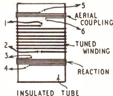
Fig. 2—Short-Wave coil
