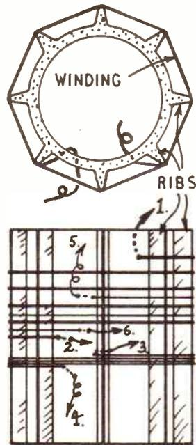
Fig. 3—S.W. coil on ribbed former
