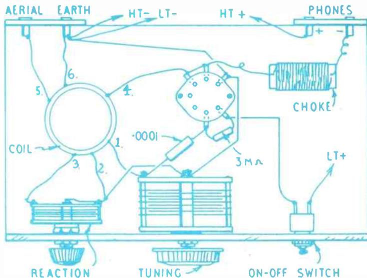
Fig. 5—Wiring plan of Fig. 4
