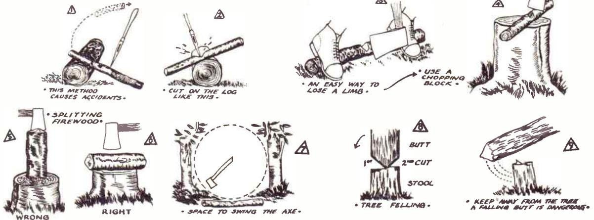
An axe is a dangerous tool in unskilled hands and should *never* be fooled with. Severe accidents have been caused by a flying axehead or an axe, on its impact with wood, suddenly rebounding at an acute angle. This disagreeable habit of the axe is the cause of many a gaping wound.
