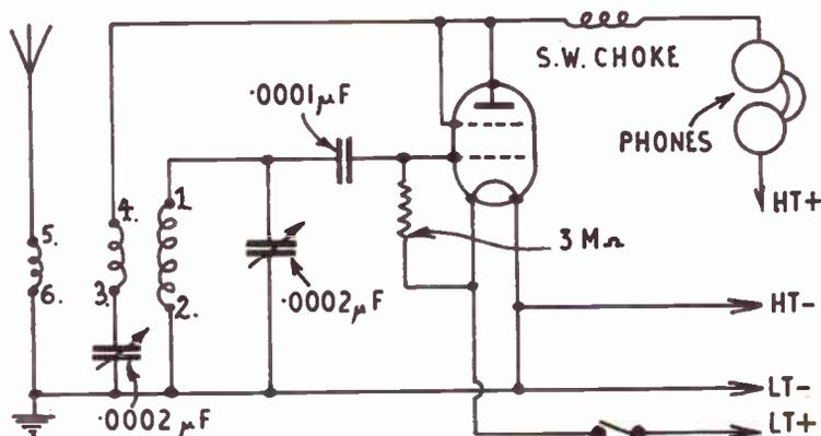
Fig. 4—S.W. 1-valve receiver
