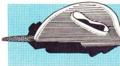
**F**ILING and rasping is much easier if this handle is used. More pressure can be applied without hurting the hands.
