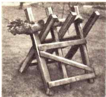
This log sawing stand described by our contributor folds flat for easy portability and has proved a big help in dealing with tree lengths.
