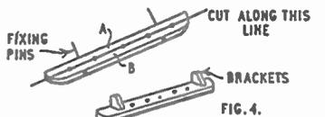
GLUE A ON HULL, FIX SHROUDS & ADD B BY GLUEING & PINNING THROUGH INTO HULL
