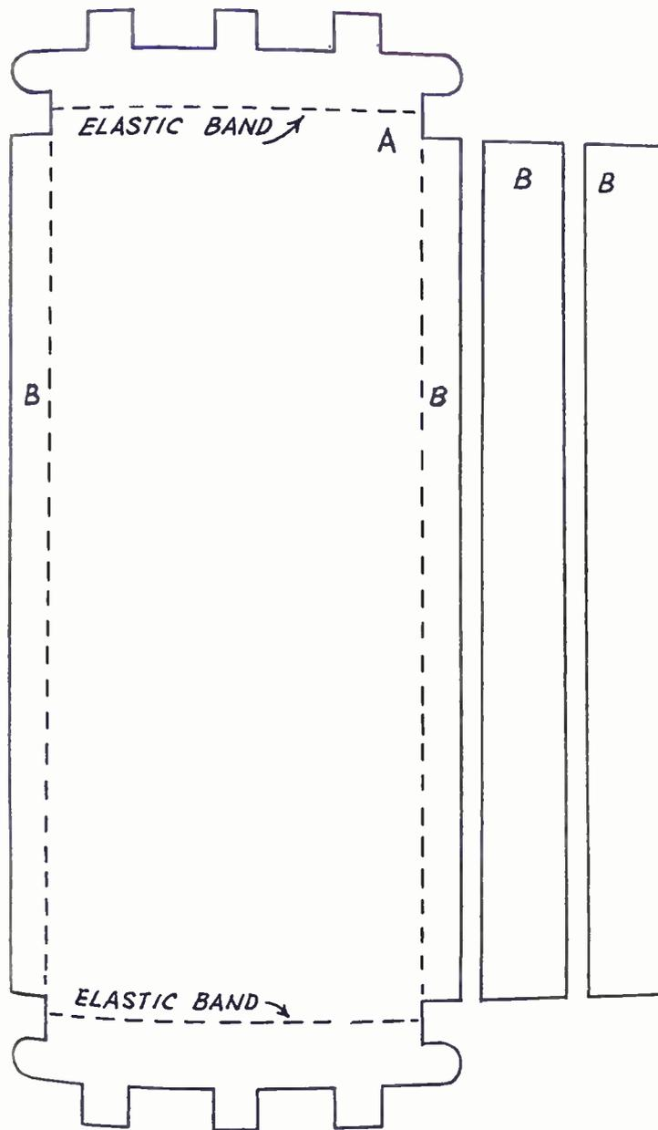
PROTECT your floats, and keep casts intact by making this handy box. Cut two of A and B from 1/2 in. wood with a fretsaw. Glue pieces B to one piece A and then hinge the remaining piece A on top. Give two coats of paint and the box is ready for use. The cast is wound round the notches, lengthwise and is held by an elastic band at each end. (M.p.)
