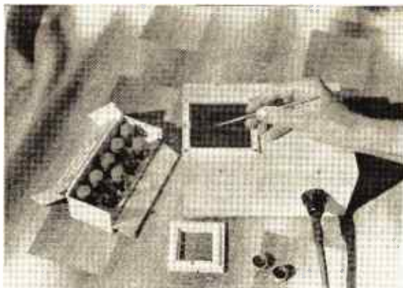
The finished illuminator, showing adaptor for 2 \times 2 slides in the foreground.
