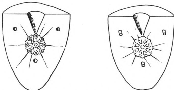
Fig. 1—The two halves of cuttlebone mould showing pour, impression, locating pins and scratches to release air
