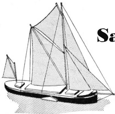
**T**HIS neat little model can be made from balsa, wire and paper. You can obtain your balsa and modelling knife from Hobbies Ltd., Dereham, or from any Hobbies branch. The parts are full size and you should cut the hull A and the bows B from  $\frac{1}{4}$  in. balsa. The hatches C, D and E are  $\frac{1}{8}$  in thick. These are cemented in the positions shown. Cut the two lee-boards F (one each side) from  $\frac{1}{8}$  in. balsa and cement in place.
