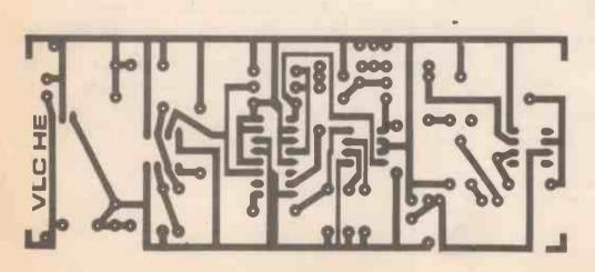
Above: The voltage level controller board
