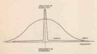
Fig. 5. Q-factor of a tuned circuit. A high-Q tuned circuit tunes sharply to one frequency, so that there is very little output at other frequencies.
