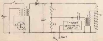
Fig 10. Basic diagram of a manual flashgun.
