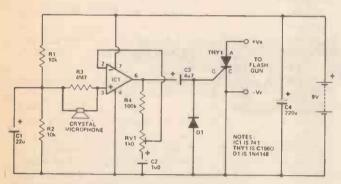
Fig. 1. The circuit diagram of the Flash Trigger.
