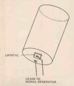
Fig. 3. An ultrasonic cleaner. The metal beaker has a piezoelectric crystal soldered to the base. Leads to the beaker and to a contact on the face of the crystal are fed with high frequency signals from a generator. The vibrations of the crystal cause the liquid in the beaker to vibrate.
