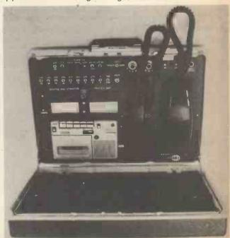
A complete anti bug system. The suitcase contains a tap detector, a tap defeater, telephone monitor and scrambler.
