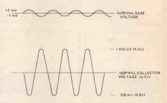
Fig. 6.8 The action of the amplifier. The wave at the output of the amplifier is an enlarged copy of the wave at the input.
