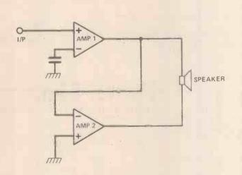
Fig. 3. Simplified internal circuitry of the HA 1388.
