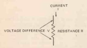
Fig. 6.2 A voltage difference caused by a current flowing through a resistor.
