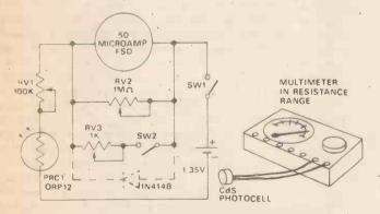
Fig. 4. Circuit diagram of a basic hand-held CdS lightmeter. This version has two ranges which are individually calibrated by RV2 and RV3.
