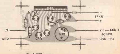
Fig. 2. PCB overlay.
