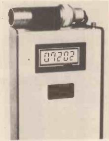
Accuracy is assured by the internal quartz controlled oscillator, typically this will be  $\pm\,1$  RPM over the range 10-100000 RPM.
