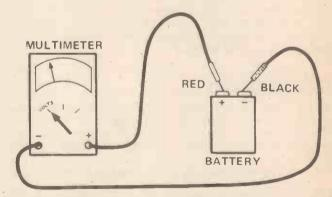
Fig. 6.3 Measuring a battery voltage. The meter must be set to a VOLTAGE range high enough to cope with the battery voltage.
