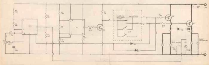
Above: Full circuit diagram of the Hazard Flasher unit.
