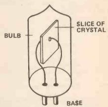
Fig. 4. A quartz crystal inside an evacuated bulb. This is a type of mounting used for crystals that control radio transmitter frequencies.
