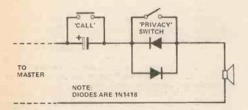
The diodes (IN1418) allow the call tone or voices from the main station to be heard but the minute voltages from the sub-station speaker are not enough to turn the diodes on.
