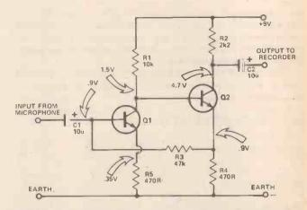
Fig. 6.7 The amplifier circuit. The figures in circles are the "design voltages" for the circuit; actual readings should not be too greatly different.
