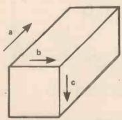
1. An isotropic crystal gives the same readings for quantities like expansivity, resistivity, etc., in any direction along the crystal, a, b, or c.
