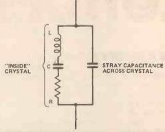
Fig. 6. Equivalent circuit of a crystal — this circuit would behave electrically just like a crystal if we could ever get suitable components for L, C and R.
