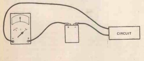
Fig. 6.5 Where to measure the collector voltage of a transistor. The meter must be switched to a voltage range as high as that used for measuring battery voltage.
