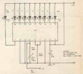
Fig 4. Circuit diagram of the LED bargraph indicator
