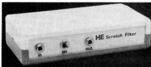
Scratch Filter — reduces the background noise of records
